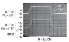
Output Waveform Driving Capacitive Load
