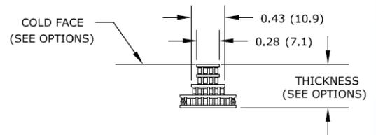
Ceramic Material: Alumina ( $\text{Al}_2\text{O}_3$ )
