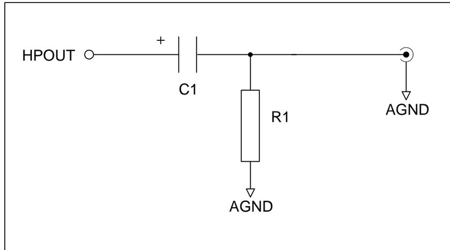
**Figure 11 Headphone Output Application Drawing**
