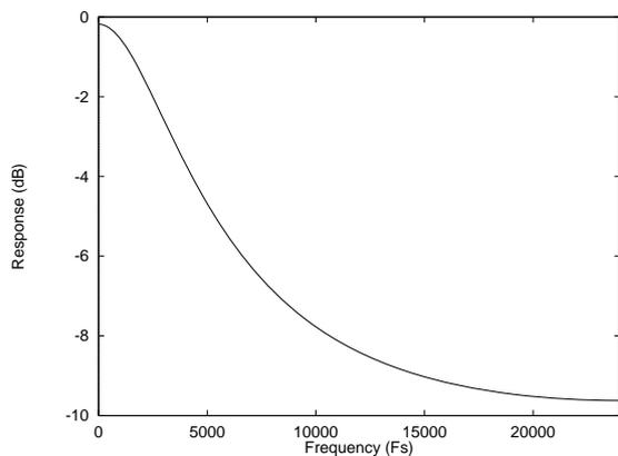
Figure 34 De-Emphasis Frequency Response (48kHz)
