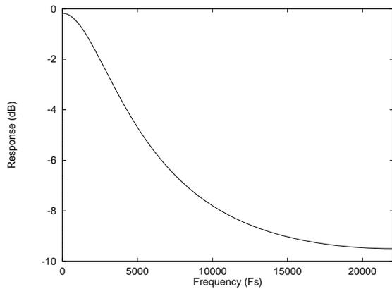
Figure 32 De-Emphasis Frequency Response (44.1kHz)
