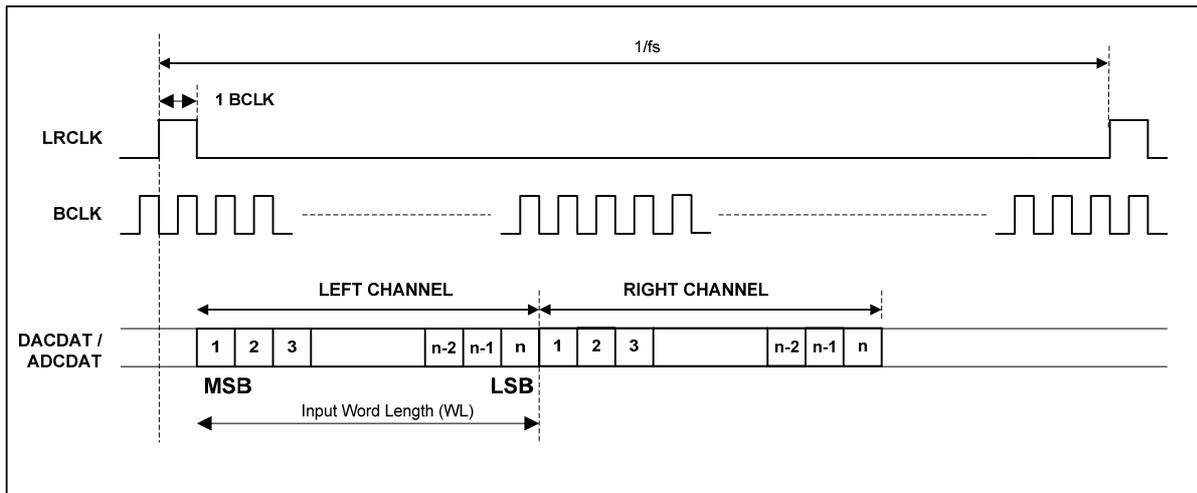
Figure 16 DSP/PCM Mode Audio Interface (mode A, LRP=1)
