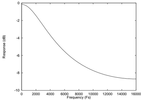
Figure 30 De-Emphasis Frequency Response (32kHz)
