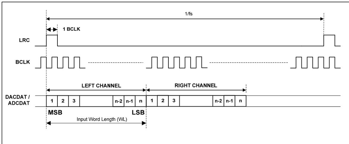
Figure 17 DSP/PCM Mode Audio Interface (mode B, LRP=0)
