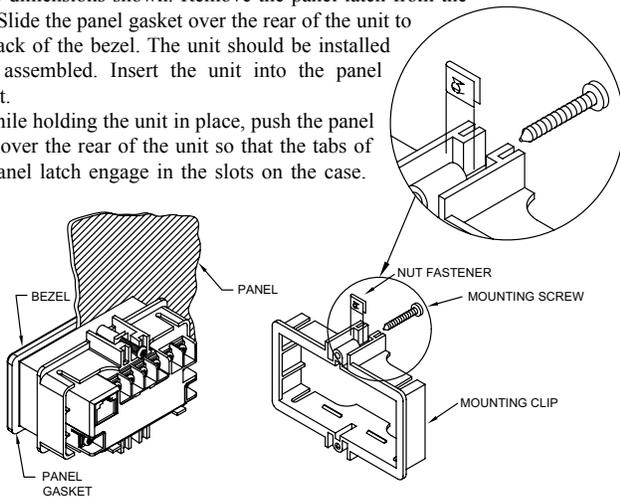
The panel latch should be engaged in the farthest forward slot possible. To achieve a proper seal, tighten the latch screws evenly until the unit is snug in the panel (Torque to approx. 28 to 36 in-oz [0.202 to 0.26 N-m]). Do not over-tighten the screws.
