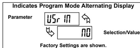
For numeric values, press the **RST** button to access the value. The right hand most digit will begin to flash. Pressing the **RST** button again increments the digit by one or the user can hold the **RST** button and the digit will automatically scroll. The **SEL** button will advance to the next digit. Pressing and holding the **SEL** button will enter the value and move to the next parameter.
