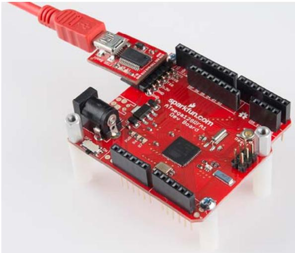
*A 3.3V FTDI Basic Board connected to the development board's serial programming header. Right-angle headers were previously soldered to the header. As a bonus, the FTDI basic can also power the dev board.*
