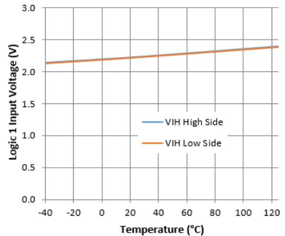
**Figure 21.** Logic 1 Input Voltage vs. Temperature
