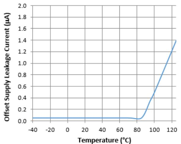
Figure 27. Offset Supply Leakage Current vs. Temperature
