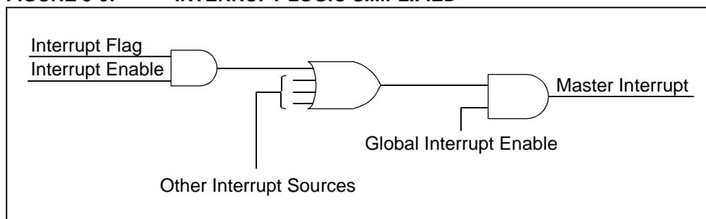
When the master interrupt line is asserted, the PICmicro finishes the current instruction, stores the next address on the CALL stack then jumps to the Interrupt Service Routine (ISR). It also clears the GIE bit, preventing another interrupt from occurring while servicing the current one.
