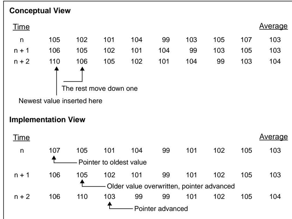
Calculating averages in a mid-range PICmicro is best accomplished by using the FSR to keep track of where the next value will be inserted. This ensures the oldest value is always overwritten with the newest and doesn't waste time moving values within the memory.
