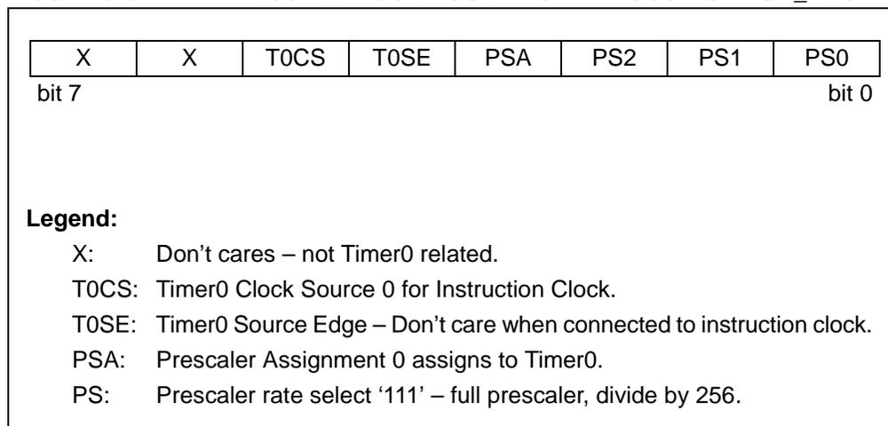
Lesson 9 configures Timer0 with the Prescaler for a maximum delay on Timer0. The prescaler will divide the processor clock by 256 and Timer0 will divide that by 256 again. Thus, Timer0 Flag will be set every 65536  $\mu$ s ( $0.0000001 \text{ second} * 256 * 256$ ), or about 15 times a second. The main program sits in a loop waiting for the rollover and when it does, it increments the display and then loops back.
