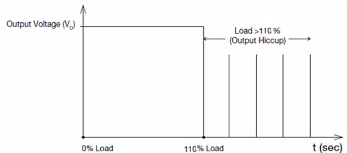
Additionally, if the  $I_o$  is  $<110\%$  but  $>100\%$  for a prolonged period of time (depending on the load), the Over Temperature Protection (OTP) will be activated due to high temperature on critical components. The power supply will then go into hiccup mode until the fault is removed; and, the input voltage is removed, then reapplied.
