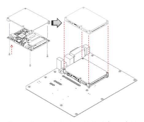
Figure 2.6 Heatspreader Pre-Assembly (For Reference Only)
