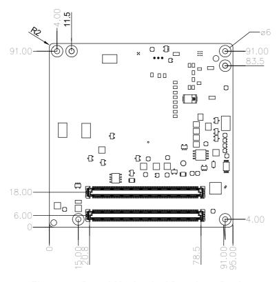
Figure 2.4 Board Mechanical Drawing - Back
