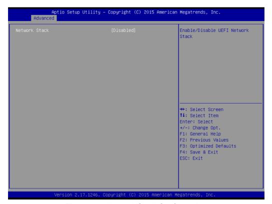
Figure 3.19 Network Stack Configuration
