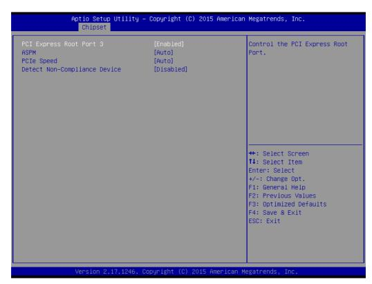
Figure 3.32 PCI Express Root Port 3 Configuration
