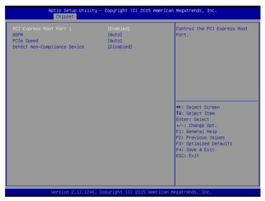
Figure 3.30 PCI Express Root Port 1 Configuration
