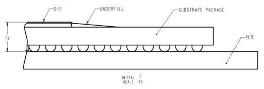
\*F5=NOM: 1.195 TOL:±0.089 (POST SMT STACKUP HEIGHT BASED ON LIMITED DATA FROM INTEL REFERENCE BOARD DESIGN)
