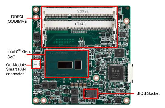
Figure 2.1 Board Chips Identify - Front
