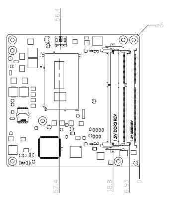
Figure 2.3 Board Mechanical Drawing - Front
