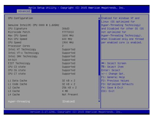
Figure 3.4 CPU Configuration
