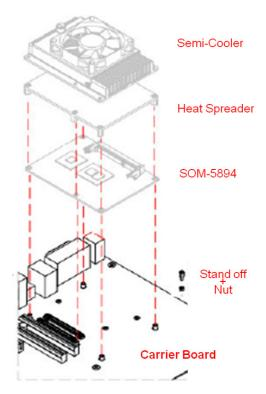
Figure 2.5 Assembly Drawing (For Reference Only)
