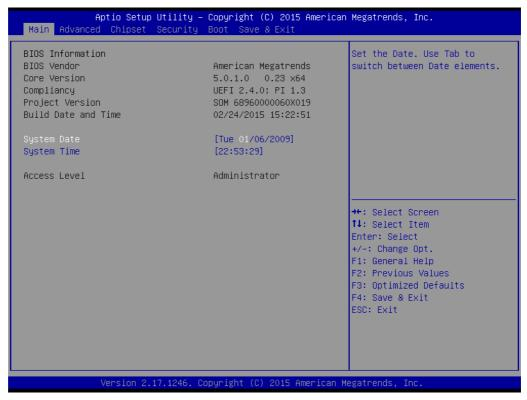
Figure 3.1 BIOS Setup Utility Main Screen
