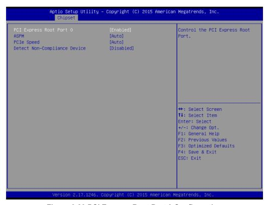
Figure 3.29 PCI Express Root Port 0 Configuration
