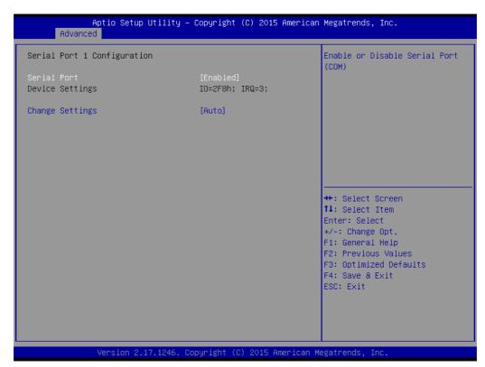
Figure 3.11 Serial Port 1 Configuration
