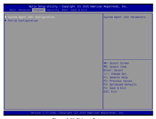
Figure 3.22 Chipset Setup
