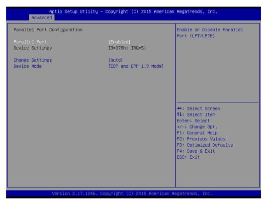
**Figure 3.12 Parallel Port Configuration**
