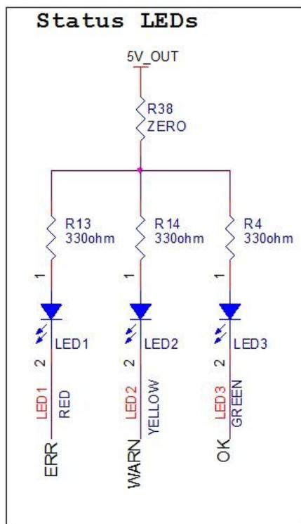
All three LEDs can be completely isolated from the rest of the Pioneer Kit by removing resistor R38, which is a 0Ω resistor. This is useful if the LEDs are not needed, but other circuits on the Shield Kit are needed. In this case, isolating the LEDs ensures that they do not interfere with other circuits that share the same pins.
