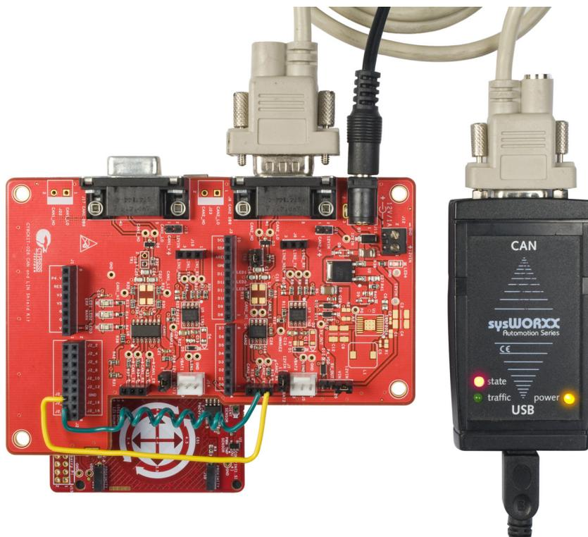
If you use a CAN bus analyzer or emulator tool to communicate with this kit, then the tool must be set up to send and receive CAN messages (at proper intervals) with proper length and message ID and at a proper baud rate.
