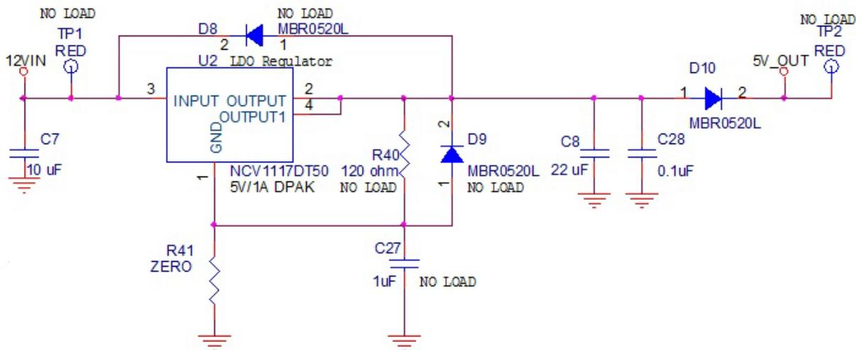
**Warning:** The regulator can support up to 1 A current, connecting this to any circuit which draws more than 1 A current will damage the regulator. Do not provide any power through the test points.
