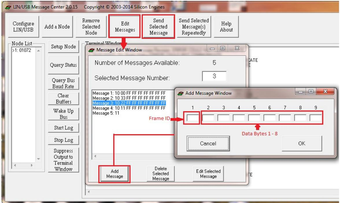
7. If a frame with ID = 0x10 is received from the master (analyzer), then the slave controls the RGB LED based on the received data command from master, as provided in Table 5-8. Note that the message must start with the ID and must contain eight data bytes even though only the first byte is used to control the LED. The other seven data bytes can be any value.
