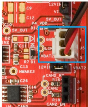
4. Connect a 12 V power supply input to the Shield Kit using any of the supply option described in [12 V Supply Input on page 25](#), and power the baseboard by populating the power selection jumper explained in [Power Selection Jumper \(J20\) on page 28](#).
