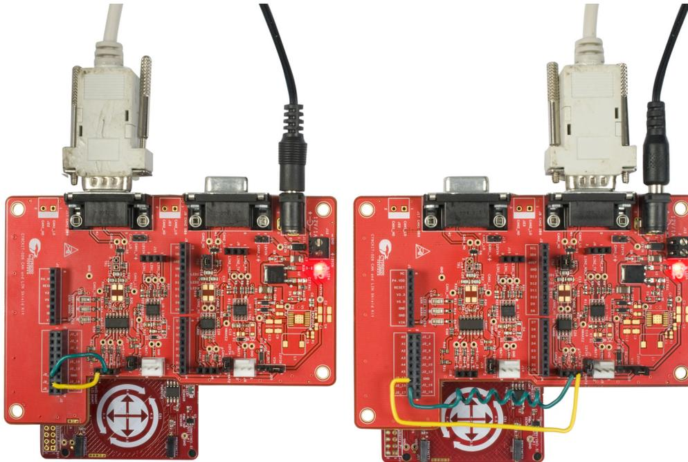
**Note:** If CAN1 is used on one kit and CAN2 is used on another kit, J10 should be removed on the kit which uses CAN2.
