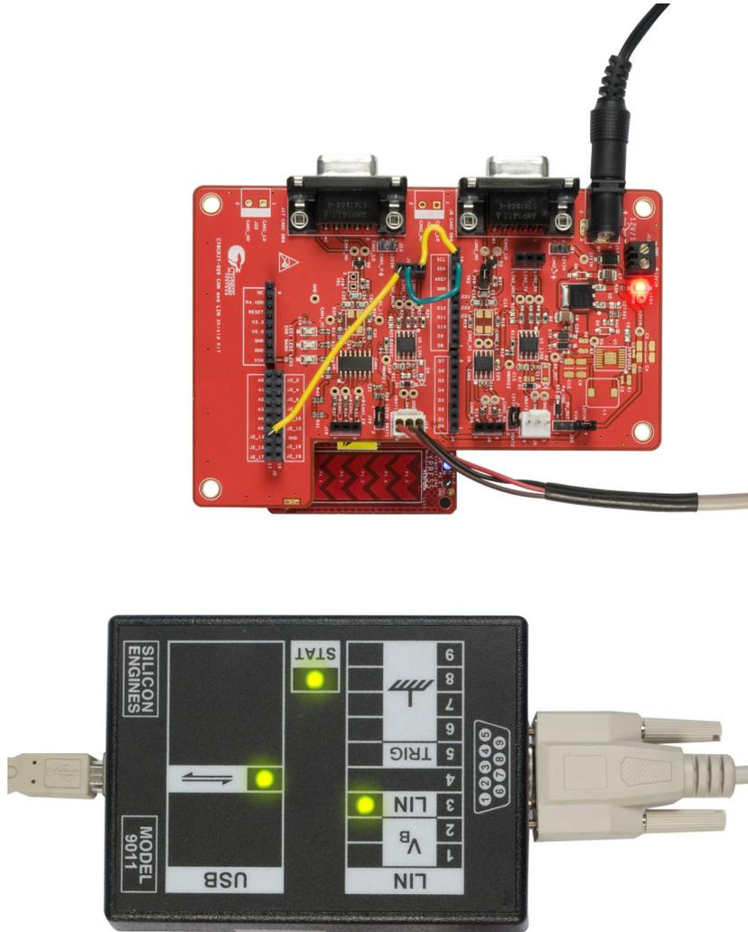
Figure 4-6. LIN Analyzer Connection to CY8CKIT-026's LIN2 Transceiver
