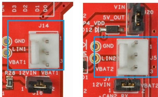
By default, the jumpers J16 and J7 are populated. These connect pin 3 (VBAT1) of the LIN1 connector and pin 3 (VBAT2) of the LIN2 connector to the VIN power rail of the Shield Kit, respectively. This is useful if you want to power up other LIN nodes/analyzers through either of the LIN connectors, or if you want to power the Pioneer Kit and shield board from the power supply (12 V) of some other LIN node (LIN analyzer).
