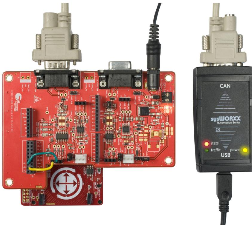
Figure 4-3. CAN Analyzer Connection to CY8CKIT-026's CAN2 Transceiver
