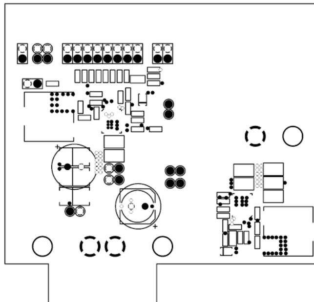
Figure 14. MIC24054 Evaluation Board Mid-Layer 1 (Ground Plane)
