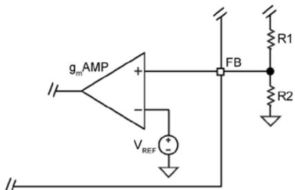
**Figure 9. Voltage-Divider Configuration**
