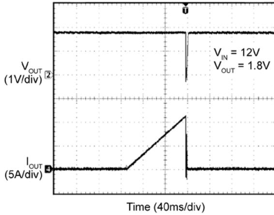
**Output Recovery Time from Thermal Shutdown**
