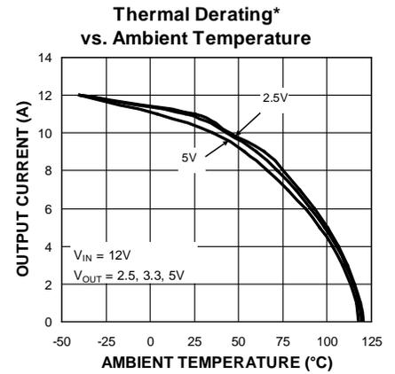
**Die Temperature\*** : The temperature measurement was taken at the hottest point on the MIC24054 case mounted on a 5 square inch 4 layer, 0.62", FR-4 PCB with 2oz finish copper weight per layer, see Thermal Measurement section. Actual results will depend upon the size of the PCB, ambient temperature and proximity to other heat emitting components.
