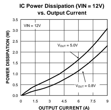
**Die Temperature\*** : The temperature measurement was taken at the hottest point on the MIC24054 case mounted on a 5 square inch 4 layer, 0.62", FR-4 PCB with 2oz finish copper weight per layer, see Thermal Measurement section. Actual results will depend upon the size of the PCB, ambient temperature and proximity to other heat emitting components.
