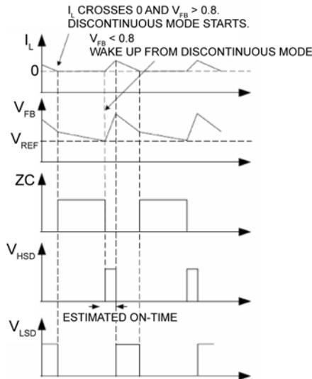
**Figure 4. MIC24054 Control Loop Timing (Discontinuous Mode)**
