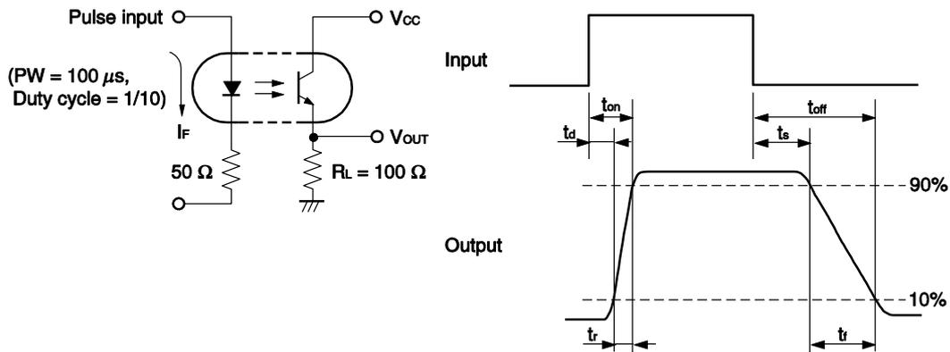
TYPICAL CHARACTERISTICS ( $T_A = 25^\circ\text{C}$ , unless otherwise specified)
