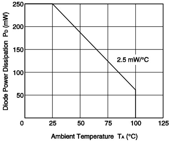
TRANSISTOR POWER DISSIPATION vs. AMBIENT TEMPERATURE
