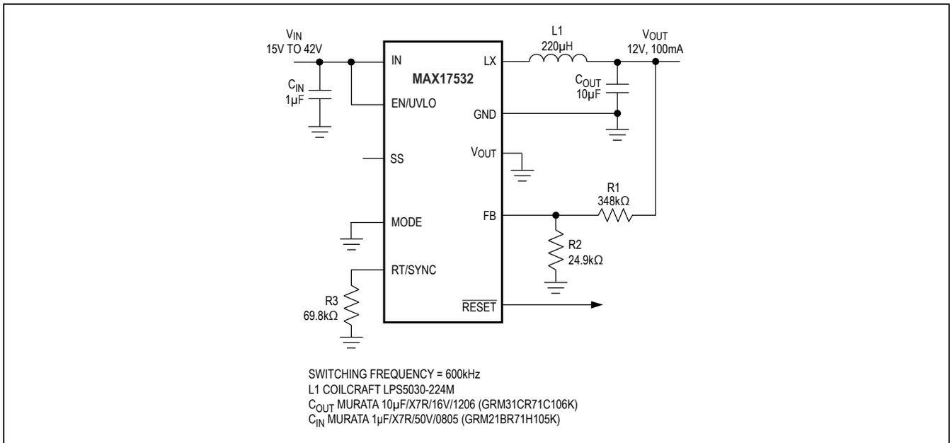
Figure 11. Small Footprint 12V, 100mA Step-Down Regulator
