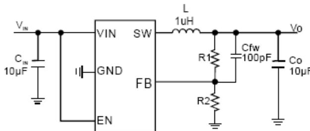
$$V_O = 0.6 \times \left( 1 + \frac{R_1}{R_2} \right)$$
