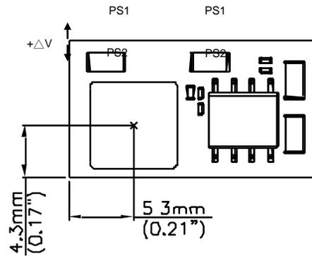
Figure 28: Temperature measurement location
