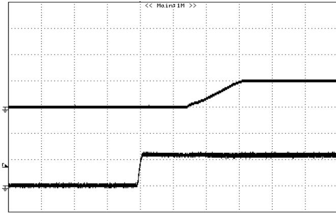
**Figure 13:** Turn on Using Input On/Off with external capacitors ( $C_o=3000\mu F$ ), 5.0V/5Aout (resistive load) (5mS/div)
