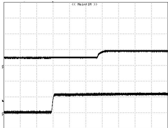
**Figure 18:** Turn on with Prebias 12Vin, 1.8V/0A out, Vbias =1.0Vdc. (5mS/div)
