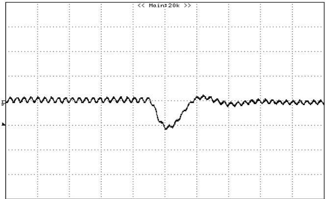
**Figure 16:** Typical transient response to step load change at 2.5A/ $\mu S$  from 50% to 100% of  $I_o$ , max at 12Vin, 5.0V out ( $C_{out}=1\mu F$  ceramic+ 10 $\mu F$  Tantalum)(200mV/div, 10 $\mu S$ /div)
