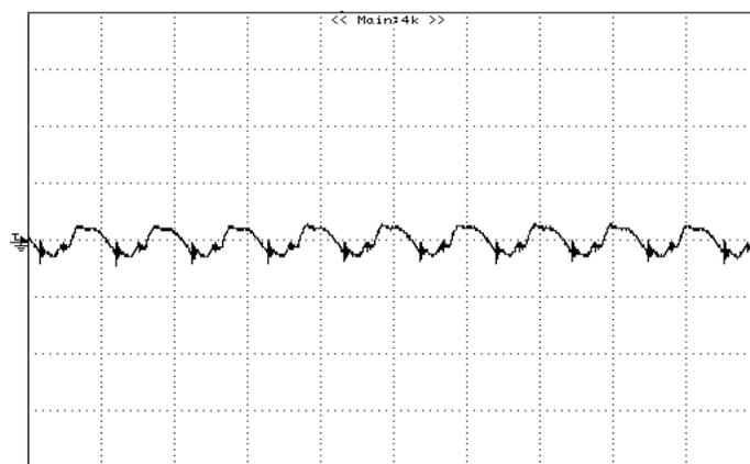
**Figure 8:** Output ripple & noise at 12Vin, 3.3V/5A out
