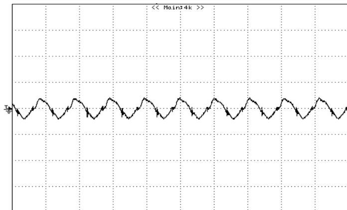
**Figure 7:** Output ripple & noise at 12Vin, 5.0V/5A out
