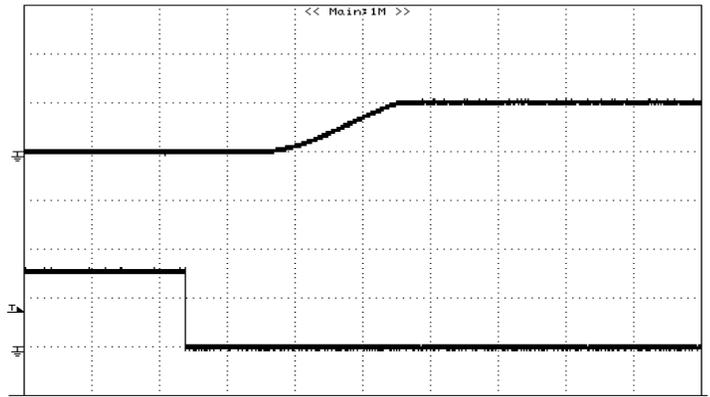
**Figure 14:** Turn on Using Remote On/Off with external capacitors ( $C_o=3000\mu F$ ), 5.0V/5A out (resistive load) (5mS/div)
