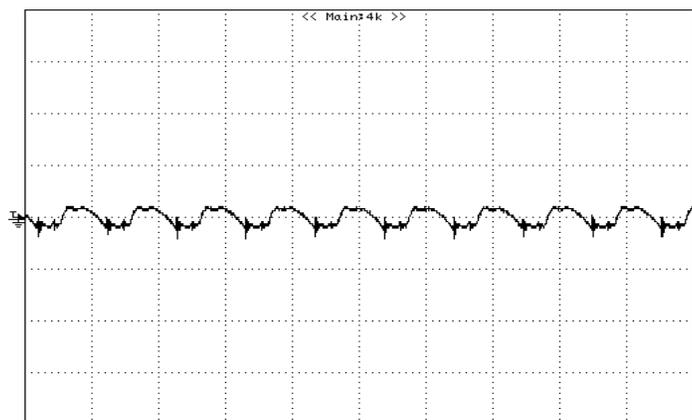
**Figure 9:** Output ripple & noise at 12Vin, 2.5V/5A out
