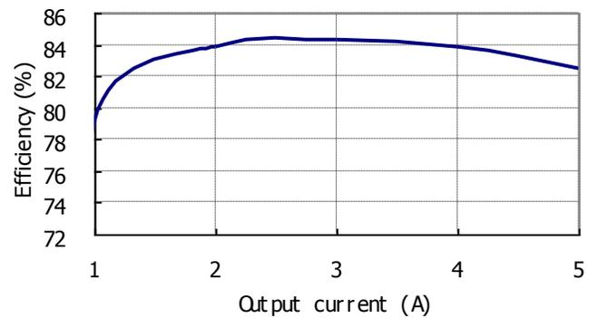
**Figure 4:** Converter efficiency vs. output current
