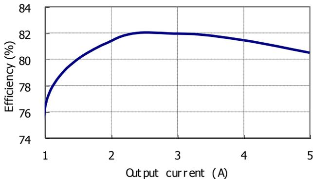
**Figure 5:** Converter efficiency vs. output current
