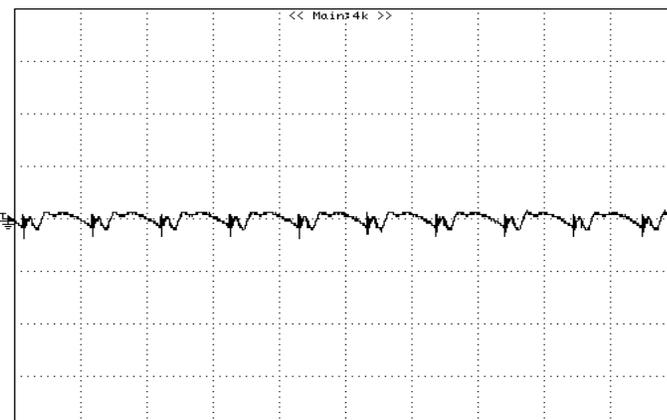
**Figure 10:** Output ripple & noise at 12Vin, 1.2V/5A out
