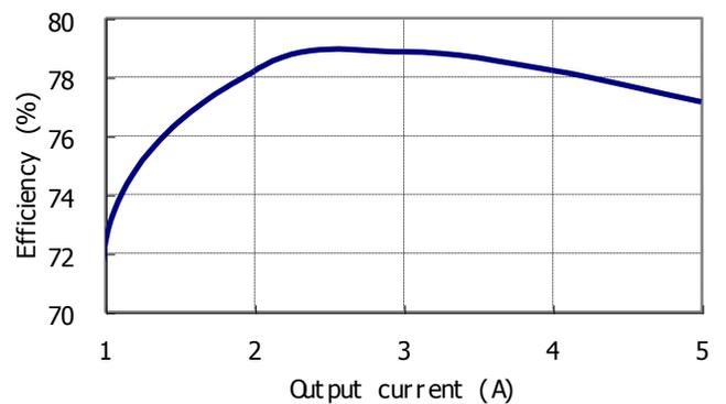
**Figure 6:** Converter efficiency vs. output current
