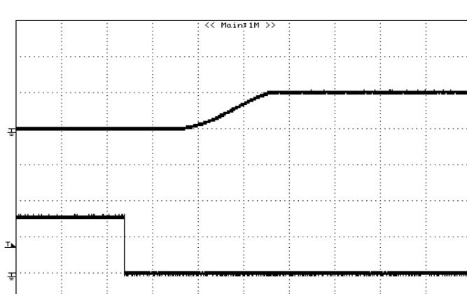
**Figure 12:** Turn on delay time at Remote On/Off, 5.0V/5A out
