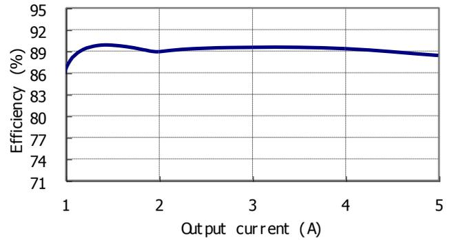
**Figure 2:** Converter efficiency vs. output current
