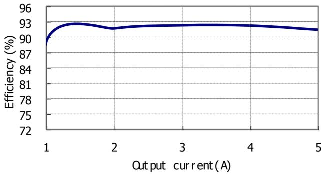
**Figure 1:** Converter efficiency vs. output current
