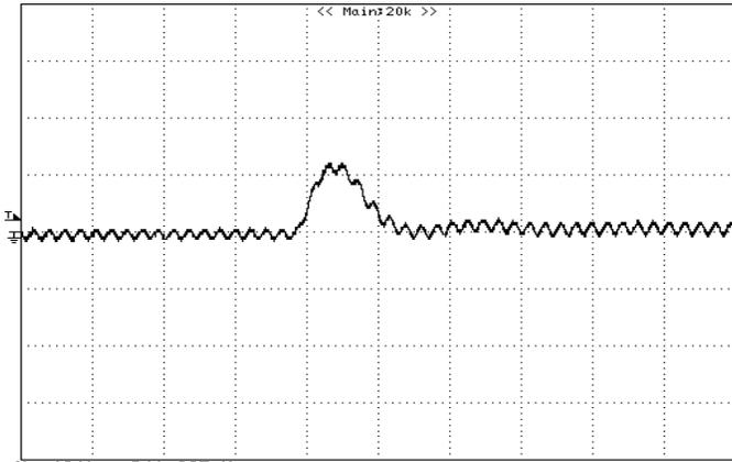
**Figure 15:** Typical transient response to step load change at 2.5A/ $\mu S$  from 100% to 50% of  $I_o$ , max at 12Vin, 5.0V out ( $C_{out}=1\mu F$  ceramic+ 10 $\mu F$  Tantalum)(200mV/div, 10 $\mu S$ /div)
