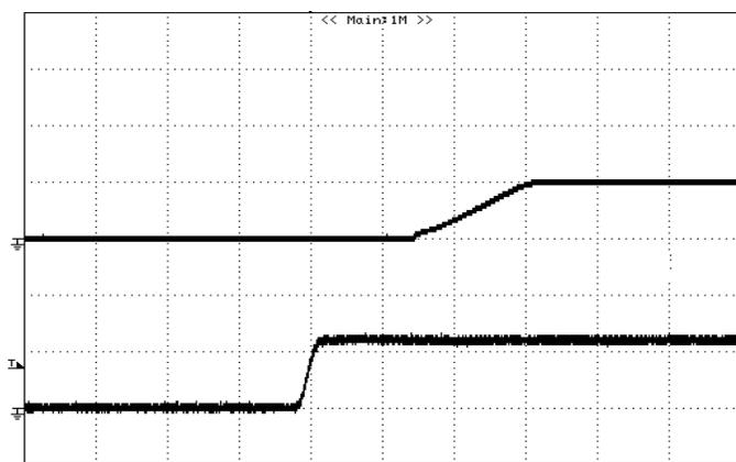
**Figure 11:** Turn on delay time at 12Vin, 5.0V/5A out
