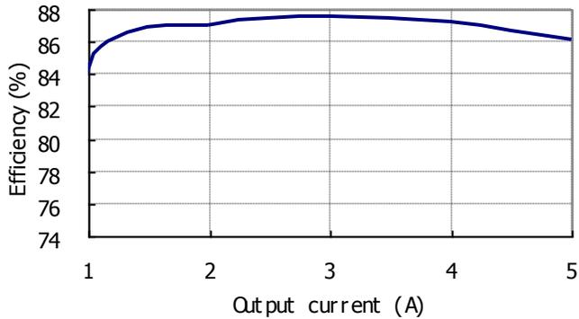
**Figure 3:** Converter efficiency vs. output current
