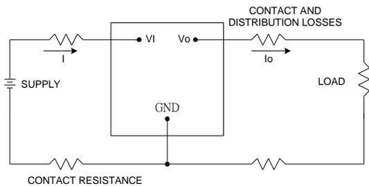
**Figure 21:** Output voltage and efficiency measurement test setup
