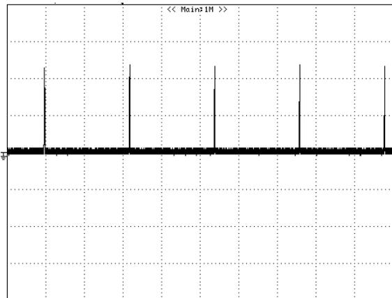
**Figure 17:** Output short circuit current 12Vin, 0.75Vout (10A/div, 50mS/div)
