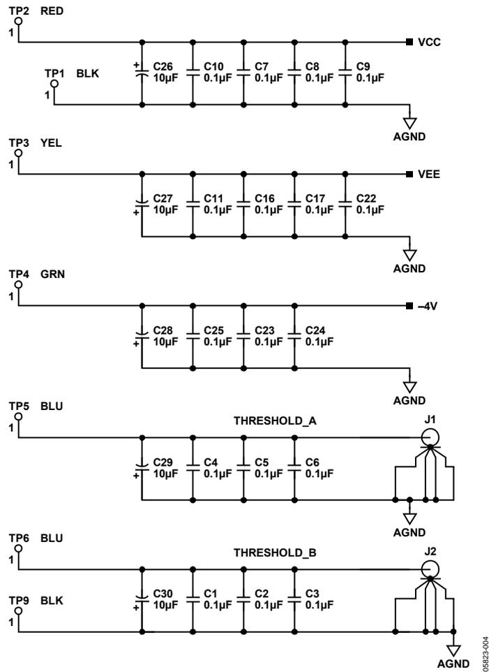
Figure 4. EVAL-ADCMP565 Schematic, Page 2 of 2
