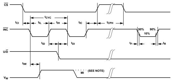
NOTE: MI IN THE AC TIMING DIAGRAM REFERS TO THE MINIMUM INCREMENTAL CHANGE IN THE  $V_W$  OUTPUT DUE TO A CHANGE IN THE WIPER POSITION.
