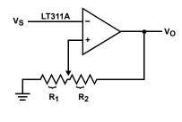
$\begin{aligned} &V_{UL} = [R_1/(R_1 + R_2)] \ V_O(max) \\ &V_{LL} = [R_1/(R_1 + R_2)] \ V_O(min) \end{aligned}$
