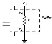
THREE-TERMINAL POTENTIOMETER; VARIABLE VOLTAGE DIVIDER
