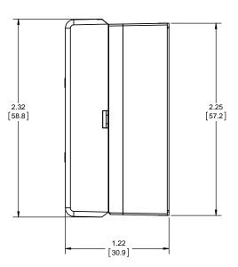
Tolerances: ± 0.02 in / 0.5 mm. All dimensions are in: inches [millimeters]
