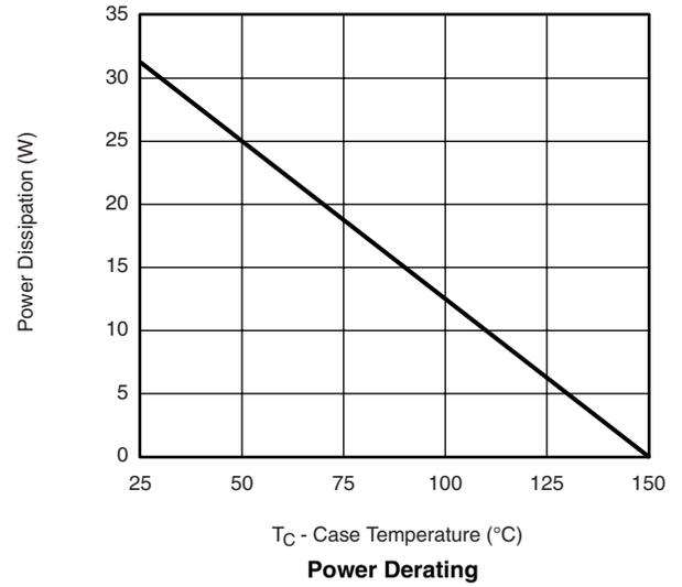
\* The power dissipation  $P_D$  is based on  $T_{J(max)} = 150$  °C, using junction-to-case thermal resistance, and is more useful in settling the upper dissipation limit for cases where additional heatsinking is used. It is used to determine the current rating, when this rating falls below the package limit.
