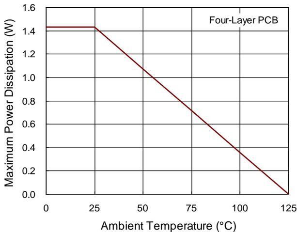
Figure 4. Derating Curve of Maximum Power Dissipation
