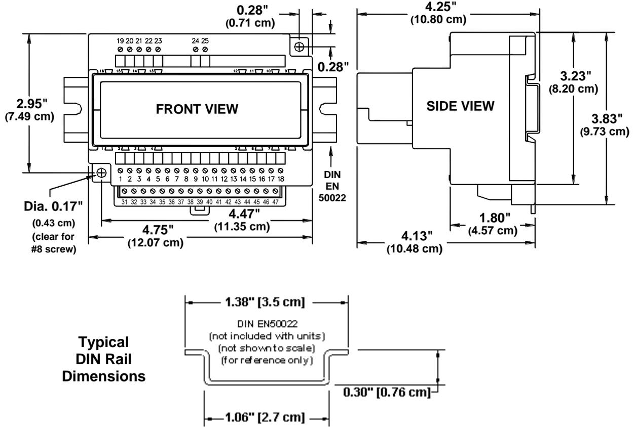
Figure 2-2 - VersaTRAK IPm2m RTU Dimensions
