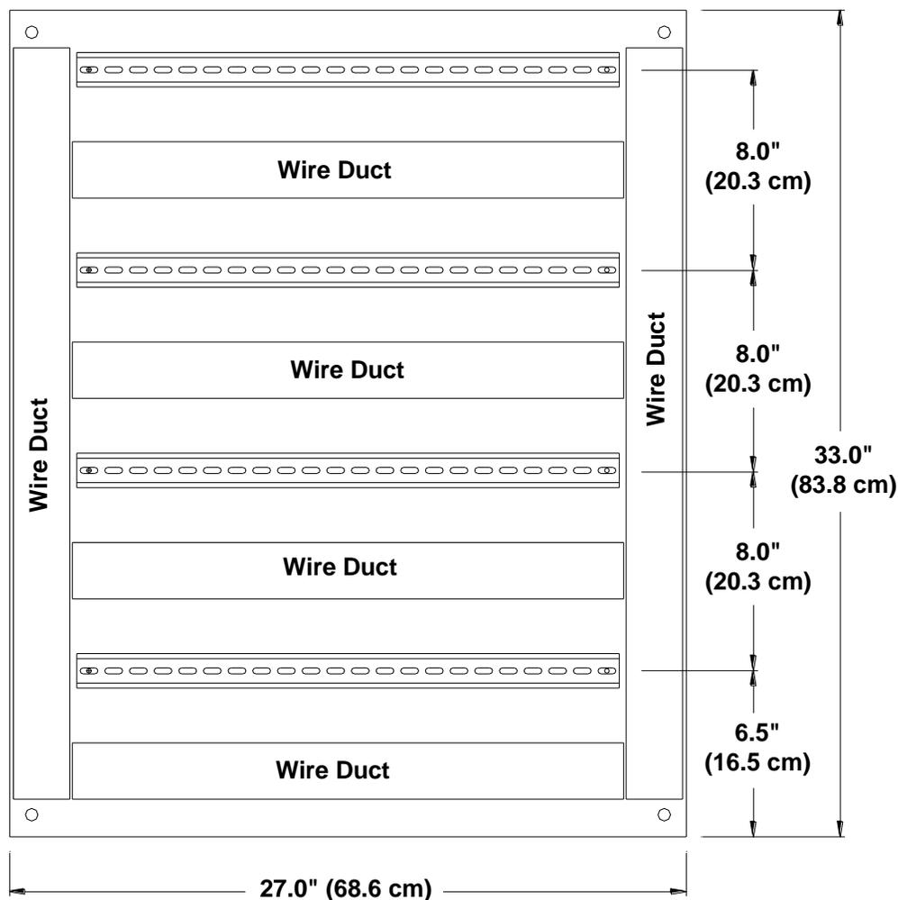
Figure 2-1 Sample Layout for a 36" x 30" Enclosure
