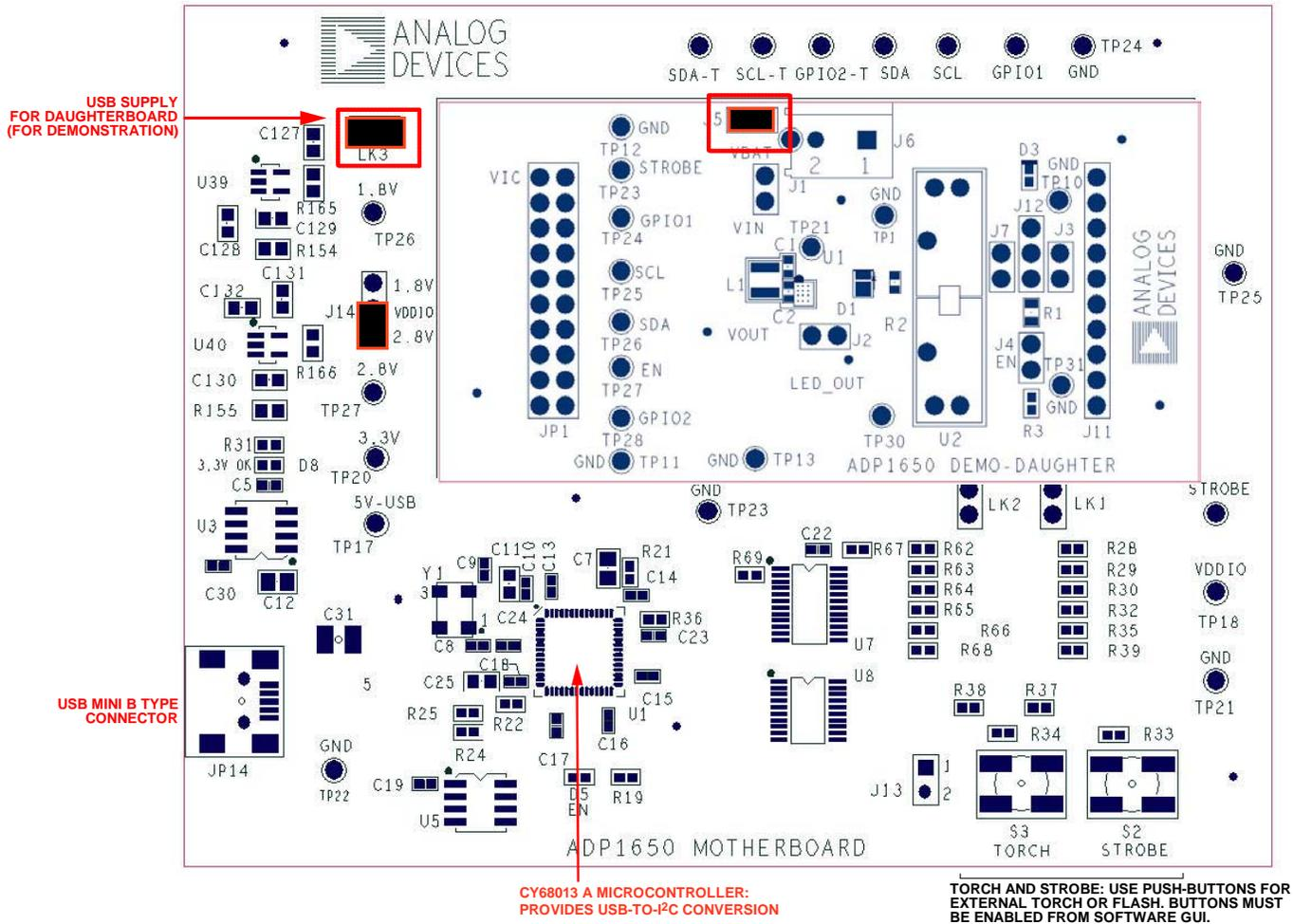
Figure 11. Powering the ADP1650 from a USB Port
