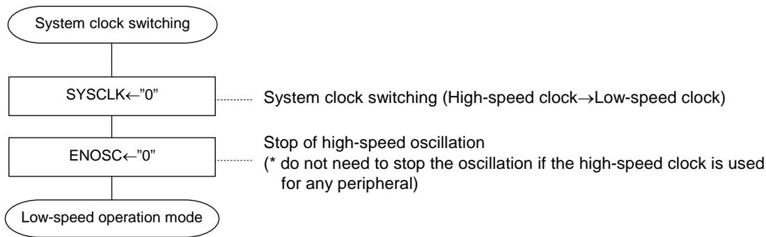
**Figure 6-7 Flow of System Clock Switching Processing (HSCLK→LSCLK)**
