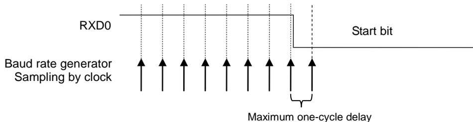
Figure 11-7 Start Bit Detection Timing (Positive Logic)
