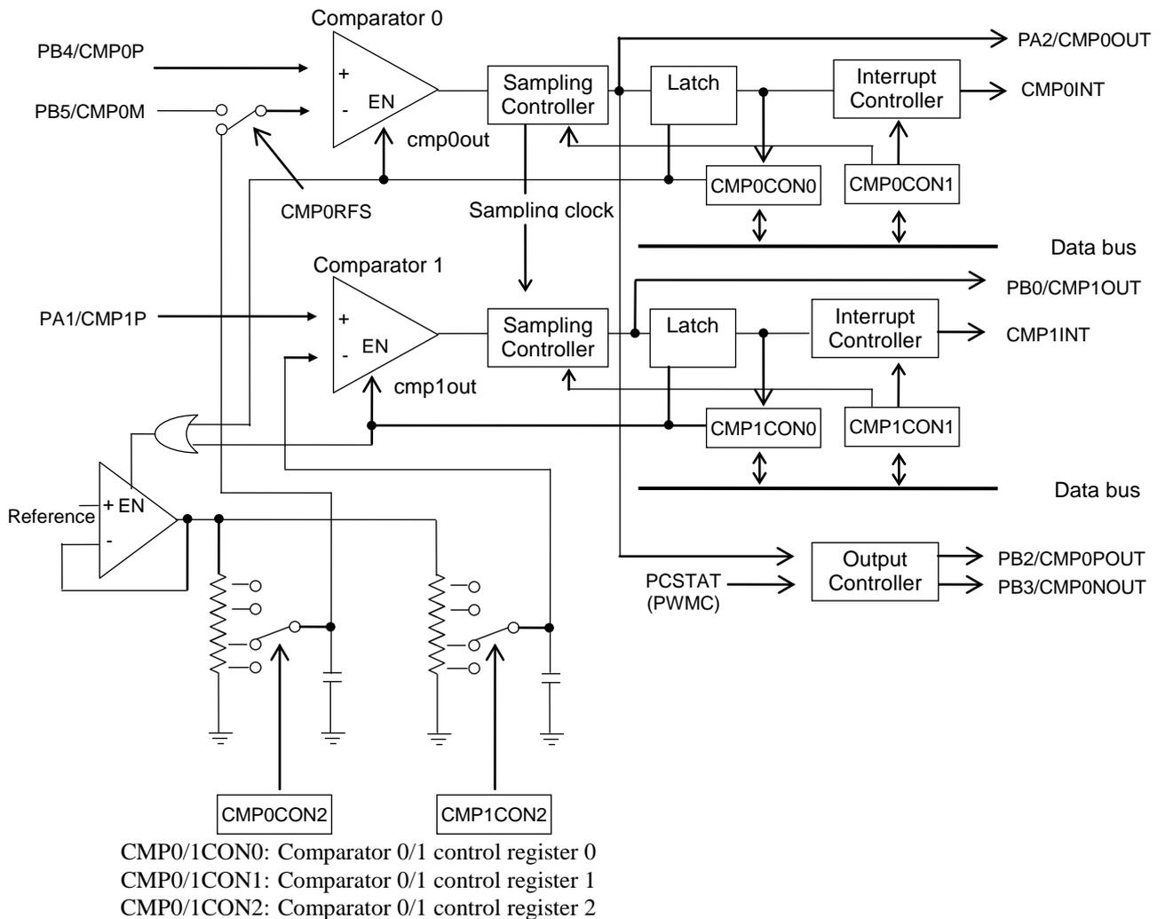
Figure 17-1 Configuration of Analog Comparator
