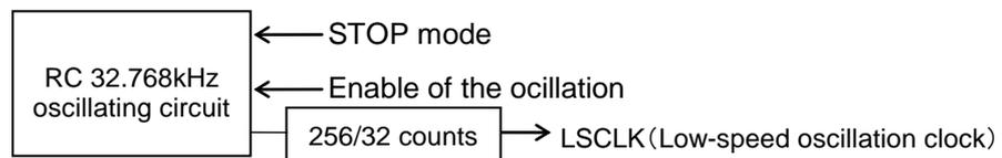
**Figure 6-2 Circuit Configuration of RC 32.768 kHz Oscillation Mode**
