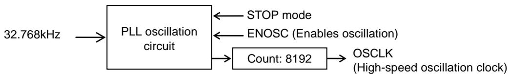
Figure 6-4 Circuit Configuration in PLL Oscillation Mode
