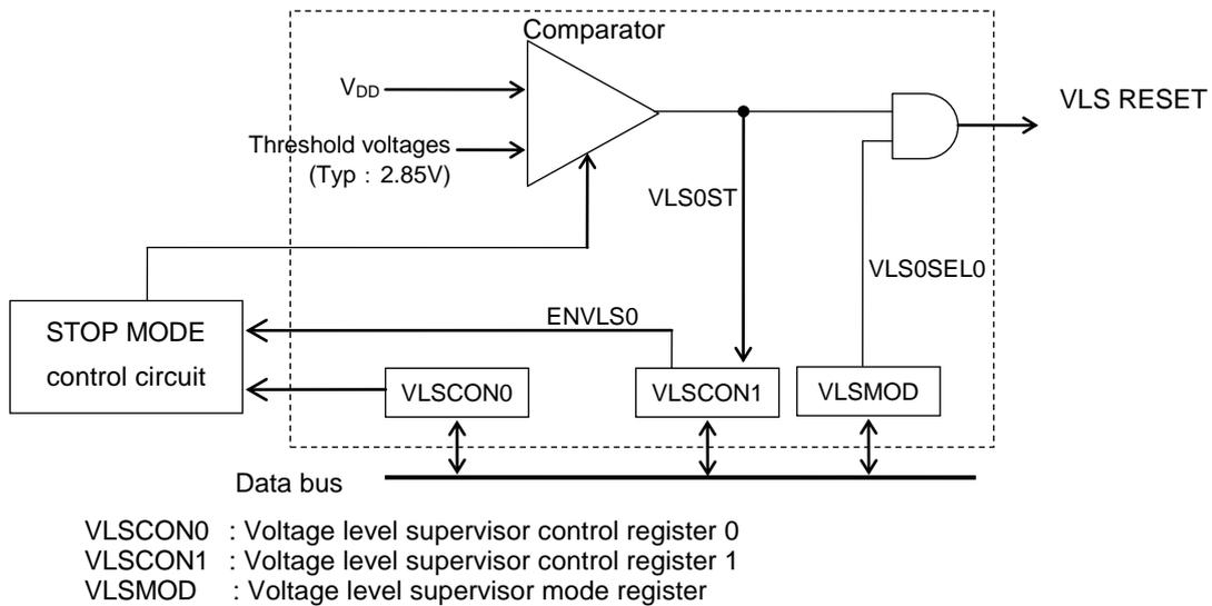
**Figure 16-1 Configuration of Voltage Level Supervisor 0**
