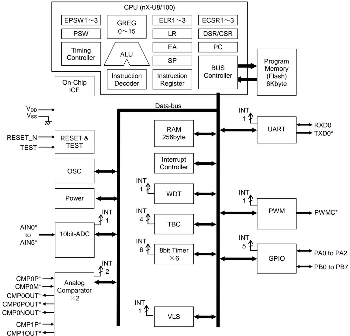
Figure 2 ML610Q102 Block Diagram
