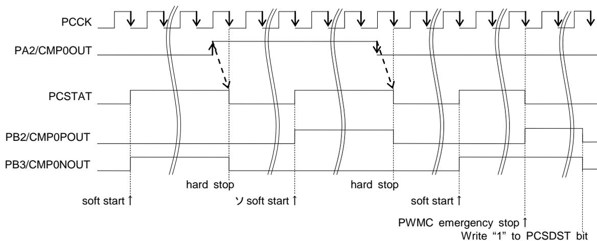
Figure 17-3 Operation Timing Diagram of CMP0POUT, CMP0NOUT
