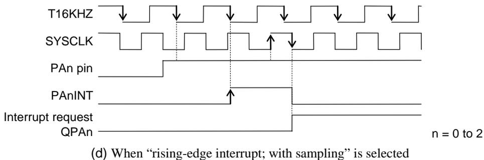
Figure 13-2 PA0 to PA2 Interrupt Generation Timing
