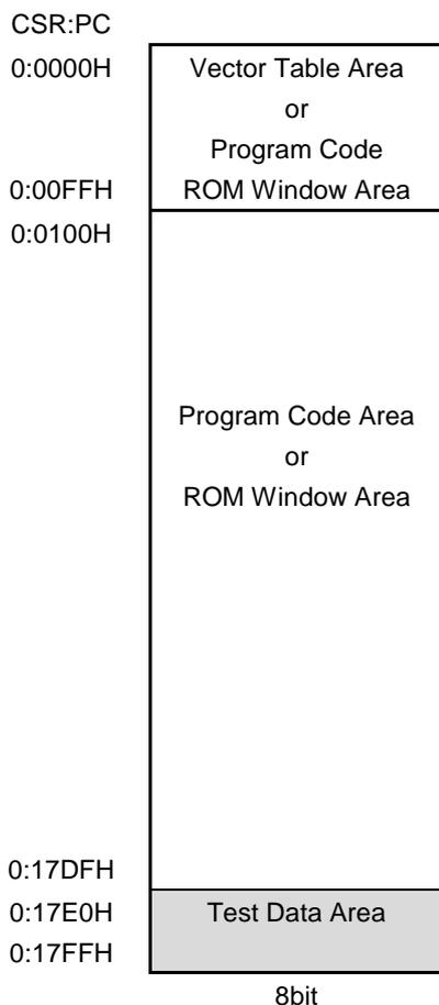
**Figure 2-2 Configuration of Program Memory Space of the ML610Q102**
