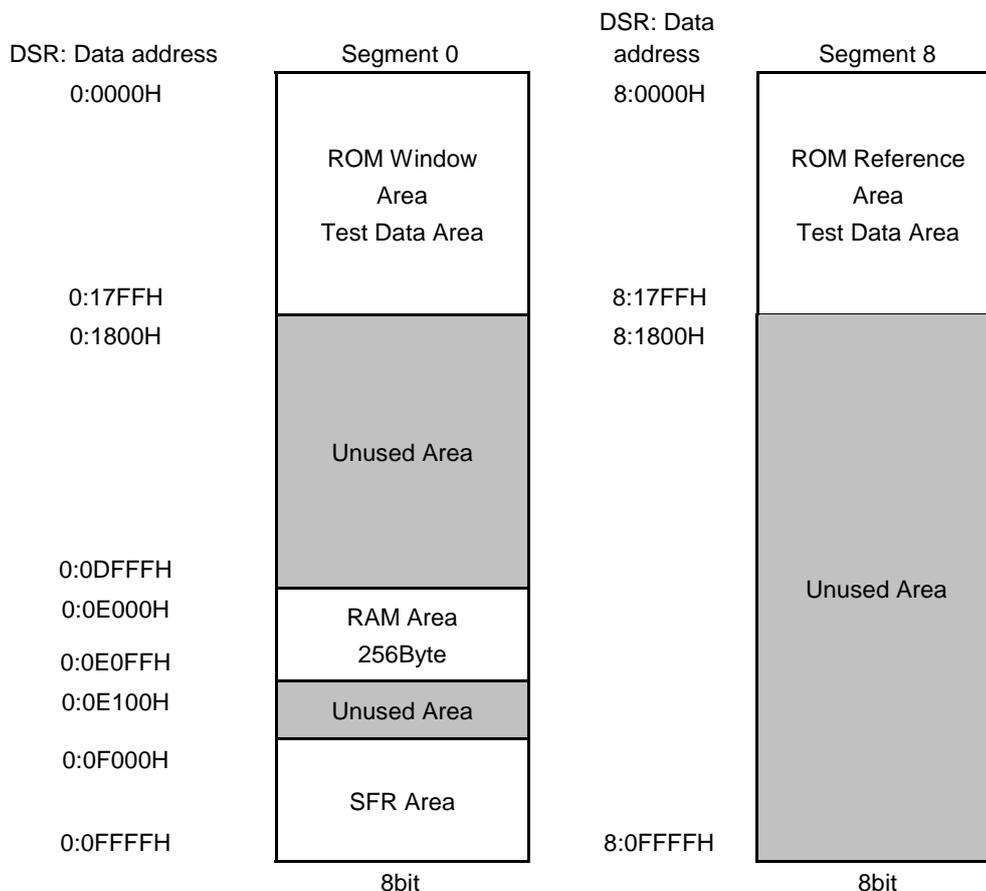
Figure 2-4 Configuration of Data Memory Space
