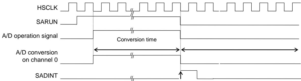
Figure 15-3 SA-ADC Operation Timing
