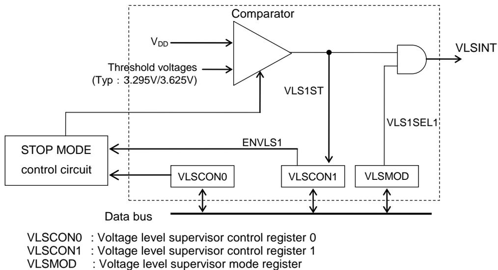
**Figure 16-2 Configuration of Voltage Level Supervisor 1**
