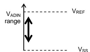
Figure 15-2 The A/D conversion pins and the conversion range
