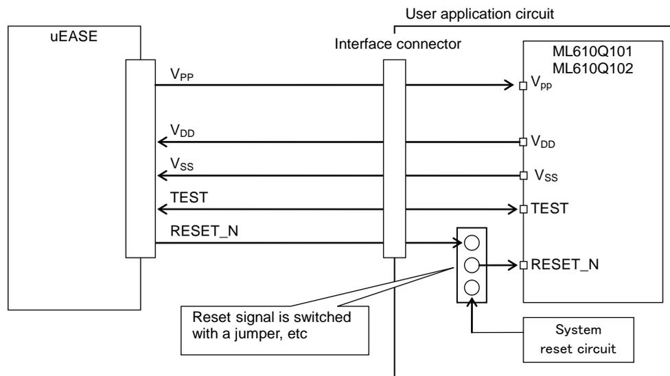
Figure 18-1 Connection to On-chip Debug Emulator (uEASE)
