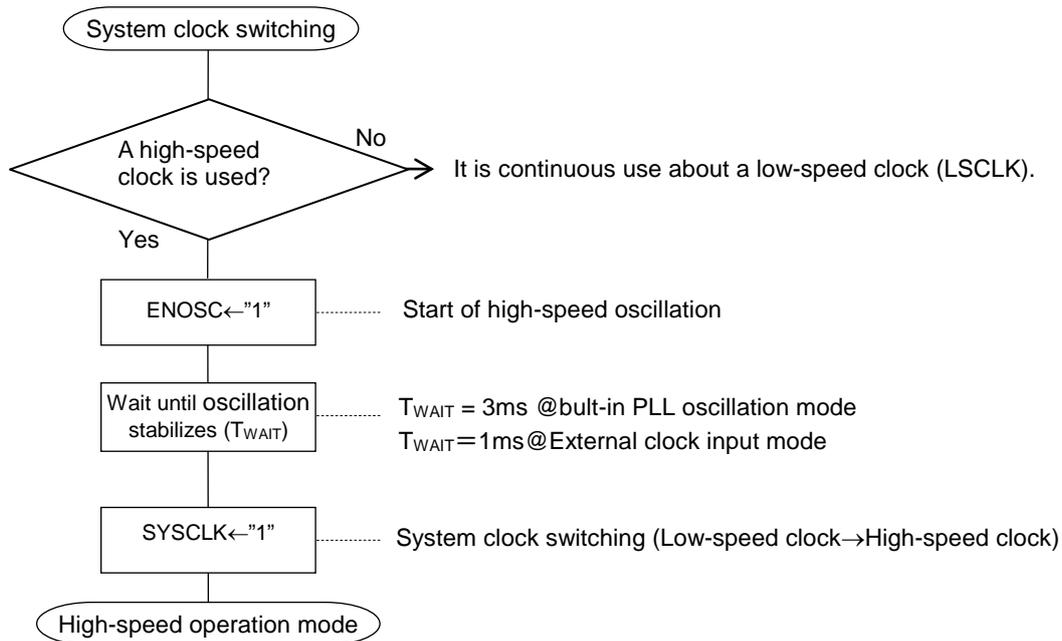
**Figure 6-8 Flow of System Clock Switching Processing (LSCLK→HSCLK)**
