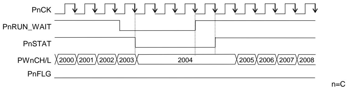
Figure 10-3 (2/2) Operation Timing Diagram of PWMC
