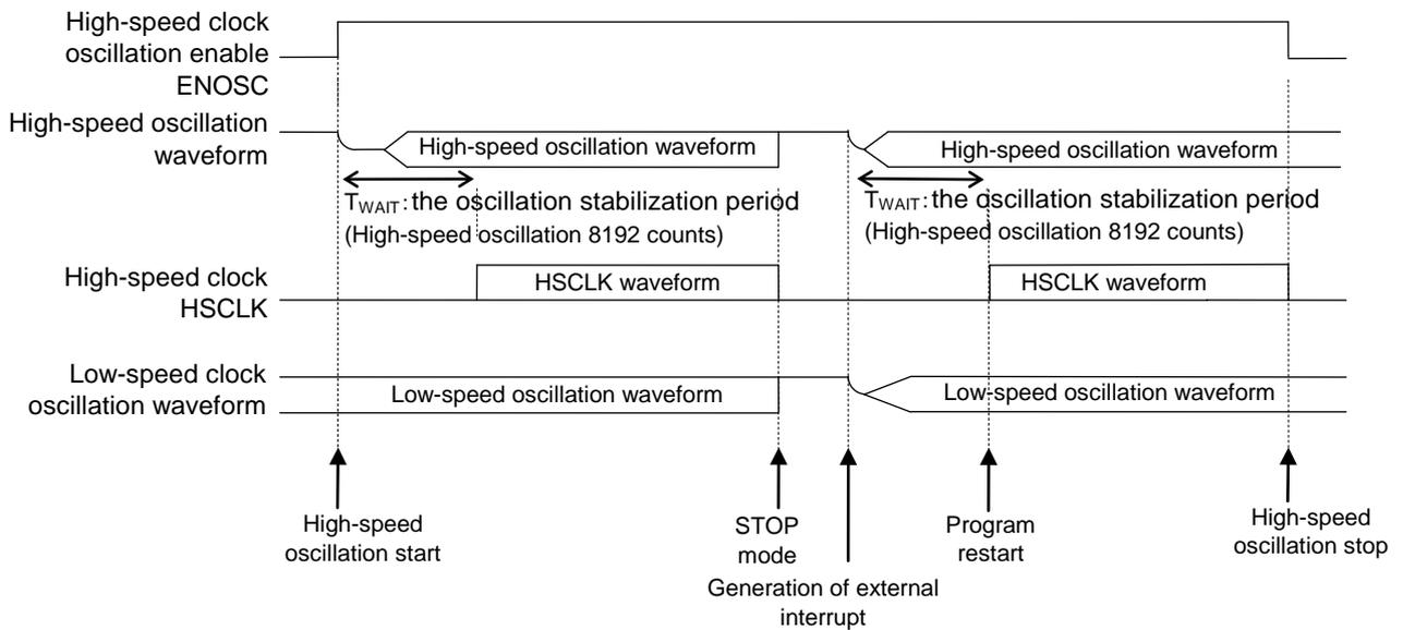
Figure 6-6 Operation of the High-Speed Clock Generation Circuit at Power-On
