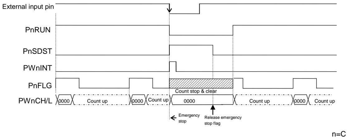
Figure 10-5 Operation Timing Diagram by Emergency Stop
