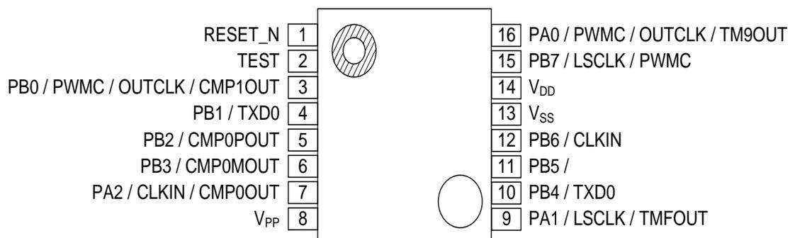
**Figure 3 Pin Layout of ML610Q101/ML610Q102 SSOP16 Package**
