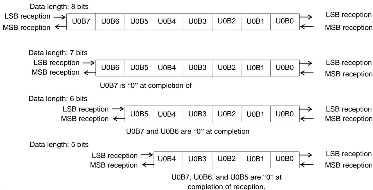
**Figure 11-4 Relationship between Transmit/Receive Buffer and Transmitted/Received Data**
