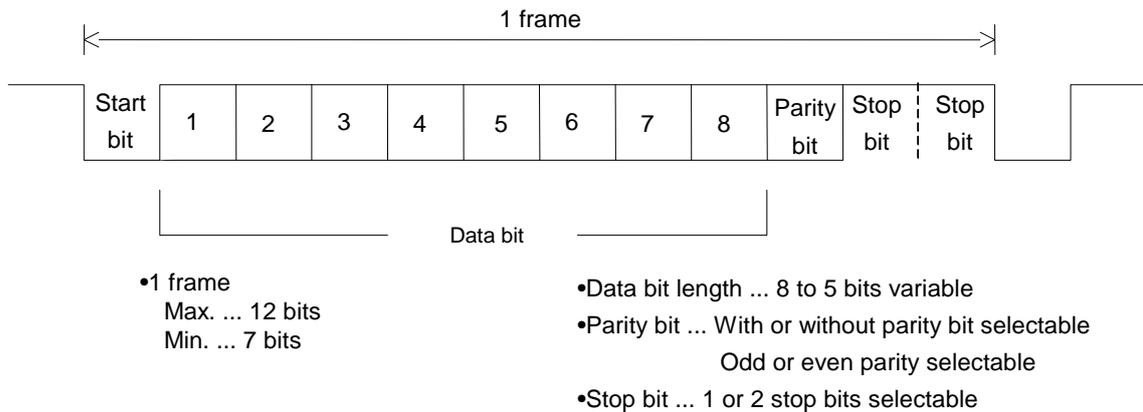
**Figure 11-2 Positive Logic Input/Output Format**
