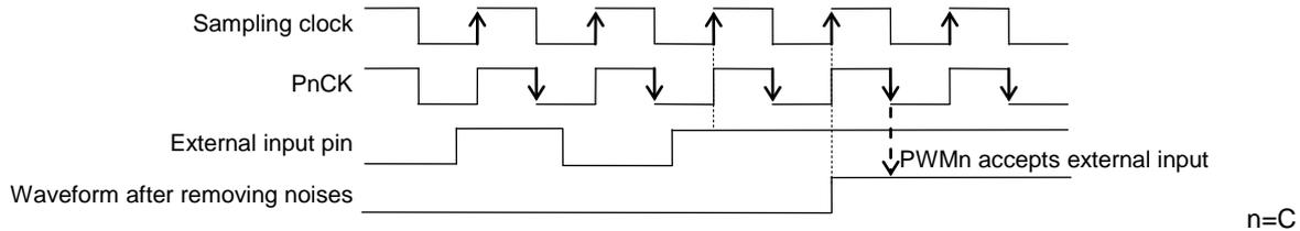
Figure 10-4 Timing Diagram of sampling of the external input
