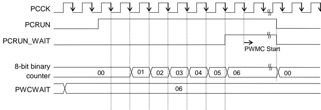
Figure 10-2 Operation Timing Diagram of PWCWAIT
