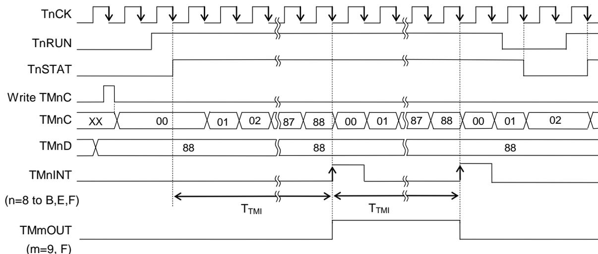
Figure 8-2 Operation Timing Diagram of Timer 8 to B,E,F
