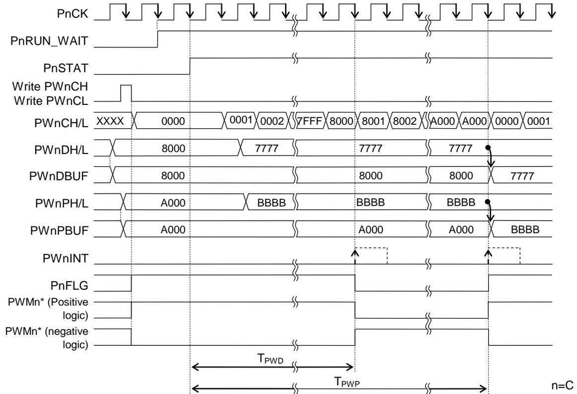
Figure 10-3 (1/2) Operation Timing Diagram of PWMC
