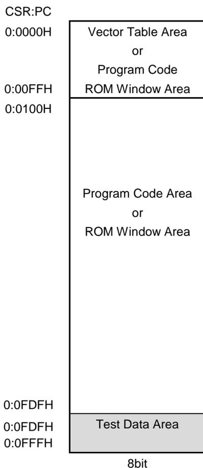
**Figure 2-1 Configuration of Program Memory Space of the ML610Q101**
