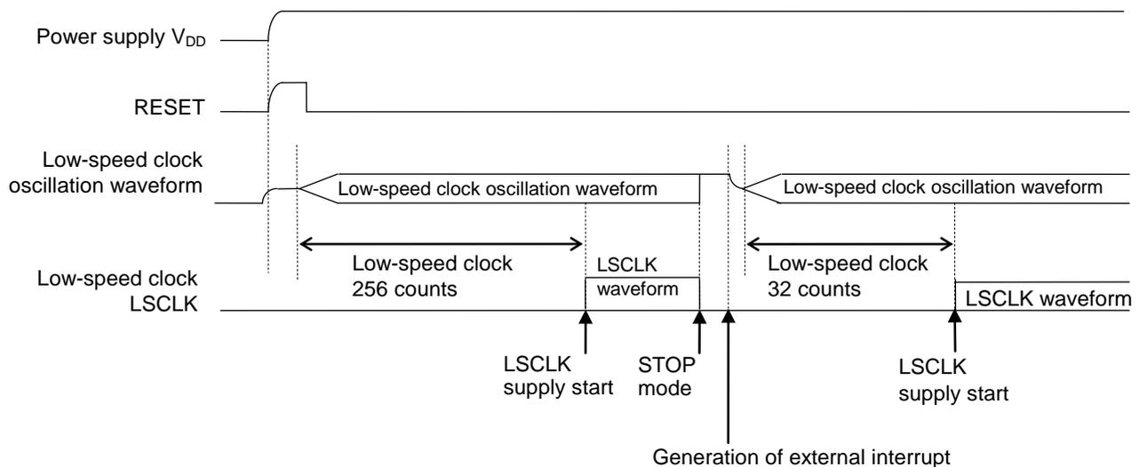
**Figure 6-3 Operation of Low-Speed Clock Generation Circuit**
