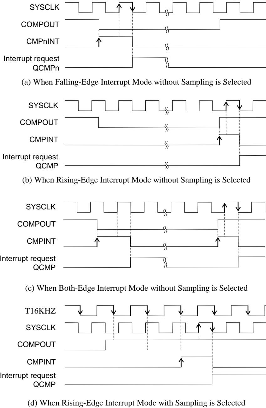
Figure 17-4 Comparator Interrupt Generation Timing
