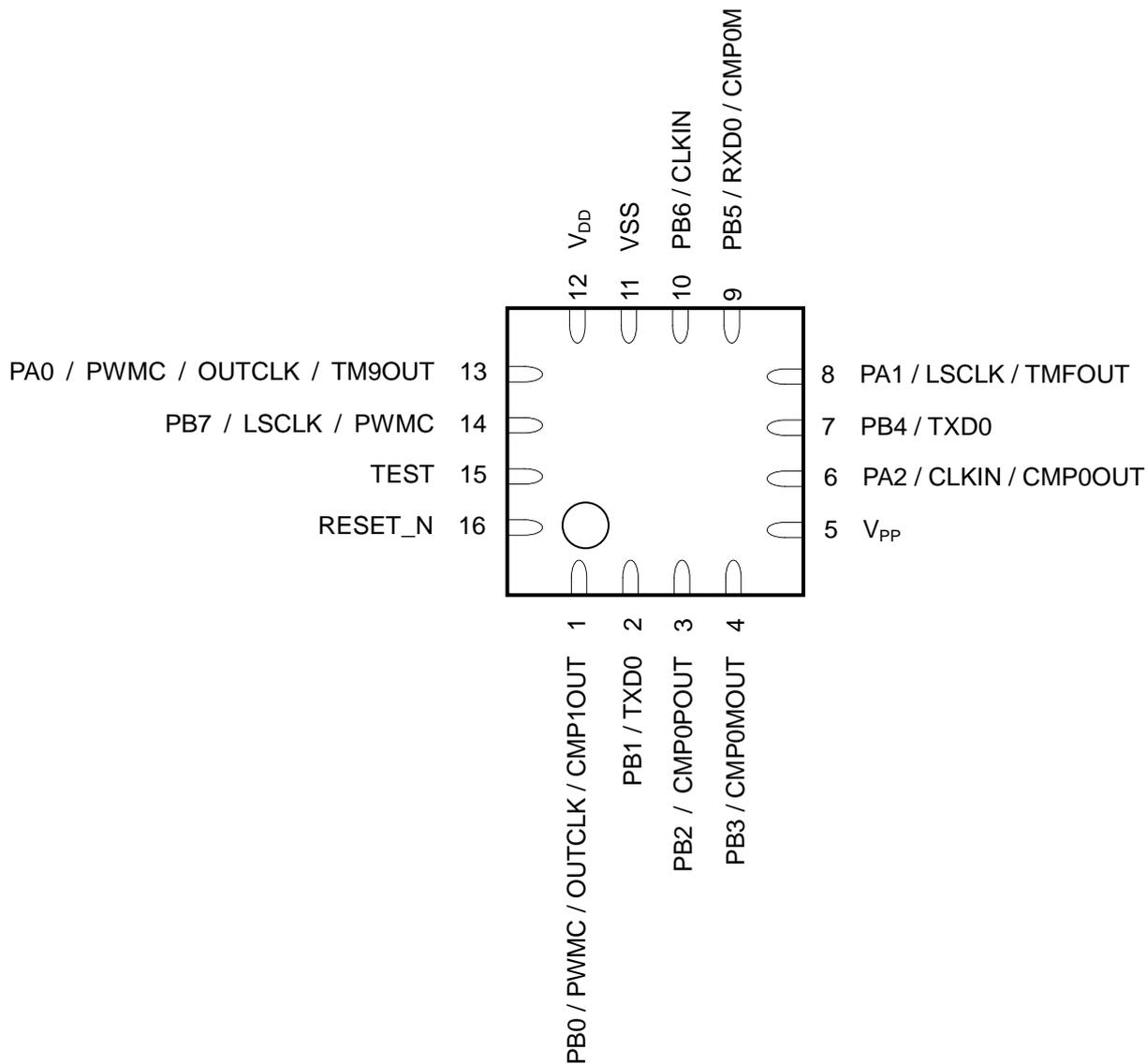
Figure 4 Pin Layout of ML610Q101/ML610Q102 WQFN16 Package
