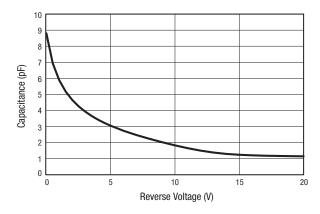
Figure 1. Capacitance vs Reverse Voltage
