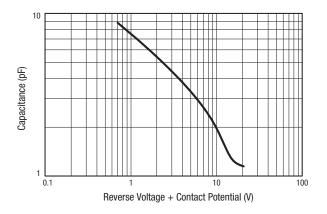
Figure 2. Capacitance vs Reverse Voltage (Logarithmic Plot)
