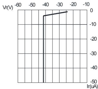
FIG.3 RED&AMBER REVERSE CURRENT VS. REVERSE VOLTAGE.
