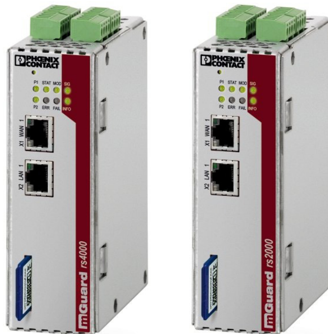
Figure 1-2 FL MGUARD RS4000/FL MGUARD RS2000
