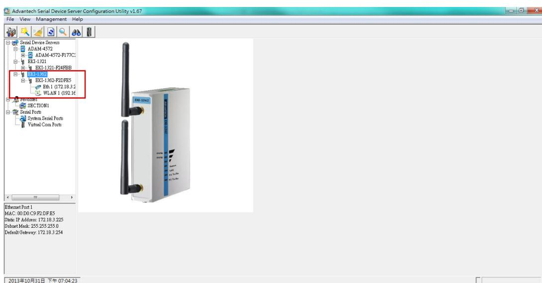
**Note!** *The default device name shown in the Configuration Utility will be the device model name appended with last 3 bytes of MAC address. You can change to a meaningful name for identification.*
