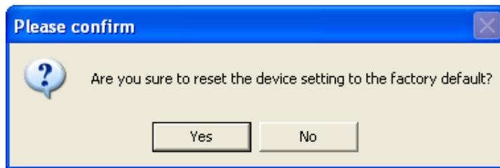
Then, please power off the serial device server within ten seconds, after reconnecting the power back, the all setting will be reset to the factory default. If the power remains more than ten seconds, the serial device server will not have any changes.
