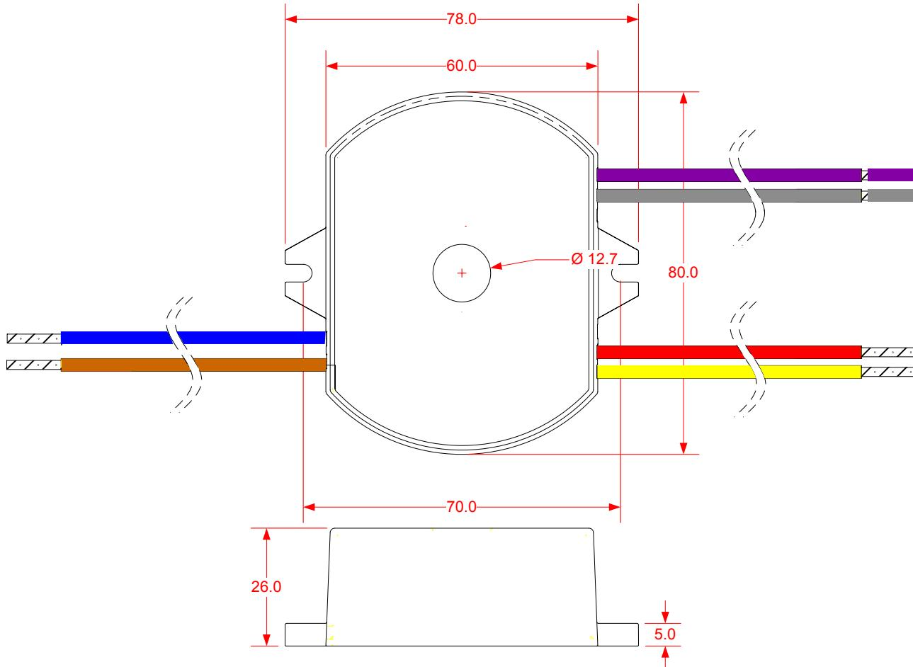
Wire length is 160mm ± 5mm, stripped 12mm ± 2mm UL1015 AWG#18 16/30 stranded 105°C Input & Output wires; AWG#22 7/30 stranded Control wires, all wires tinned. Please insure the wire nuts are installed correctly to prevent intermittent operation. Connecting the AC input to Control or Output wires will result in damage to the module. Hole in center, mounting tab slot width 4mm.
