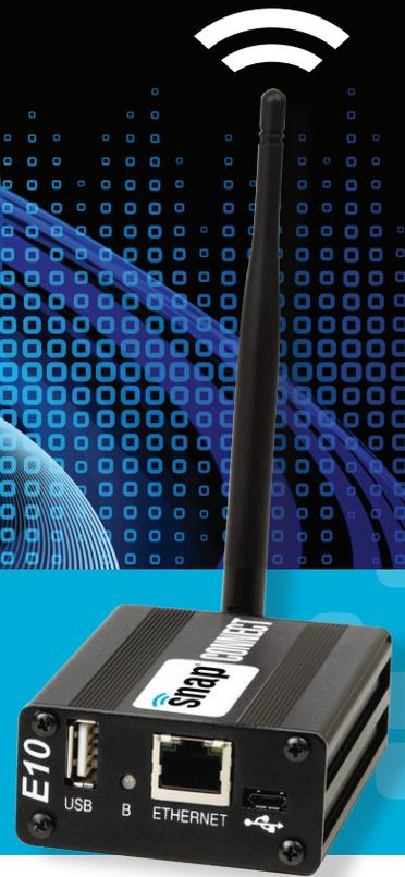
The **SNAP® Connect E10** is a rugged, powerful, embedded connectivity appliance built to interface directly with SNAP mesh networks. The E10 can collect data from SNAP devices for centralized storage, database processing or application monitoring, making it extremely easy to view or control devices over the Internet. The E10 bridges SNAP networks across TCP/IP.
