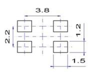
Do not design any conductive path between the pattern
