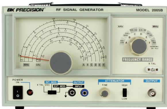
The 2005B supplies sine wave outputs from 100 kHz to 150 MHz (harmonics usable to 450 MHz) at up to 100 mV (RMS). The output can be amplitude modulated with an internal 1 kHz signal or with an external audio signal up to 1 V (RMS). An external crystal can be plugged in for precise frequency control. The output is provided via a BNC female connector.
