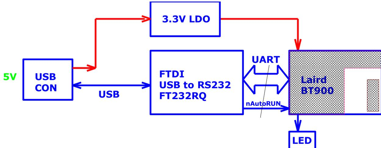
Figure 1: BT900-US block diagram
