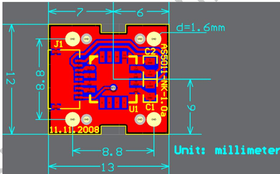
Figure 7: AS5011\_NK\_1.0 navigation module PCB, bottom view
