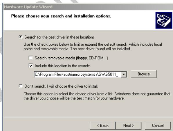
Enter the path: C:\Program Files\ austriamicrosystems AG\AS5011\_Mouse\Driver, where the Silnt.sys file is located.
