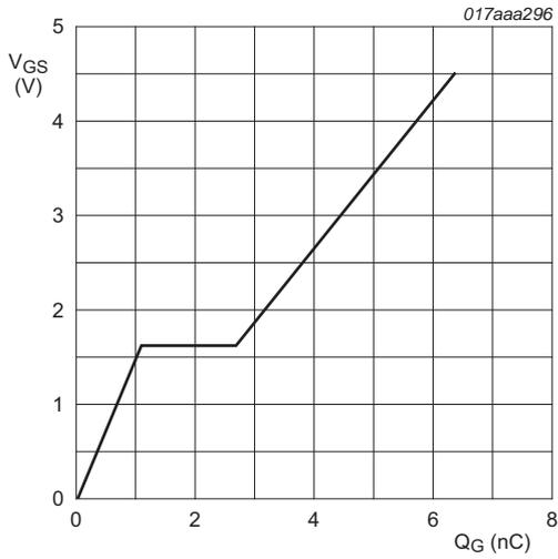
$I_D = 6.0$  A;  $V_{DS} = 10$  V;  $T_{amb} = 25$  °C
