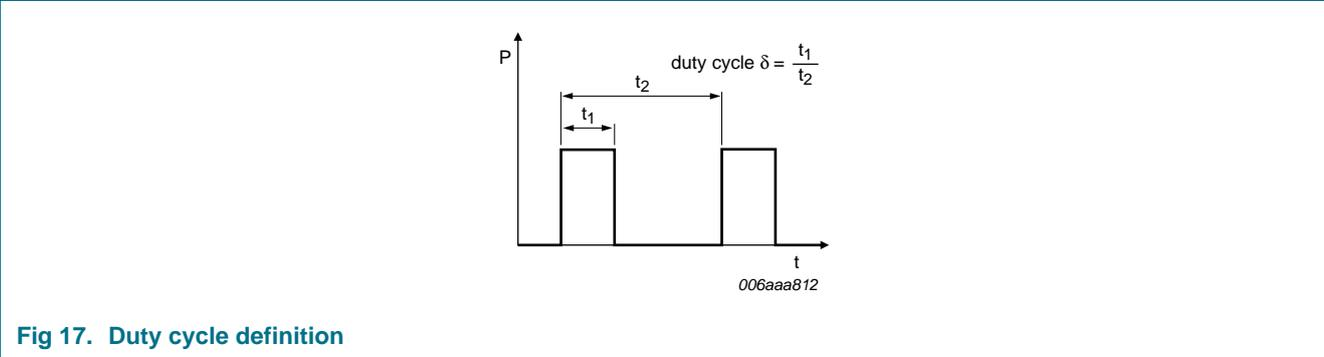
Fig 17. Duty cycle definition
