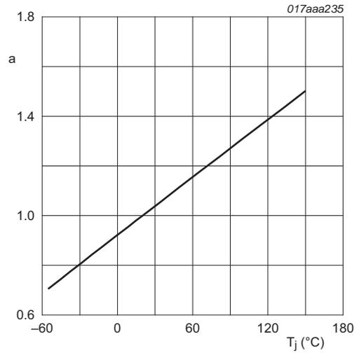
$$a = \frac{R_{DSon}}{R_{DSon(25^\circ C)}}$$
