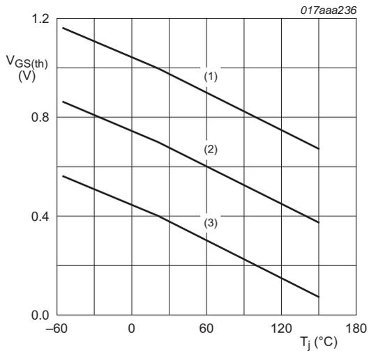
$I_D = 0.25\text{ mA}; V_{DS} = V_{GS}$
