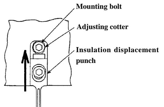
**4.1 Replacing the Insulation displacement punch**
