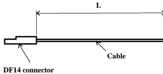
For twist cables, cut them so that cut ends are flush with each other.
