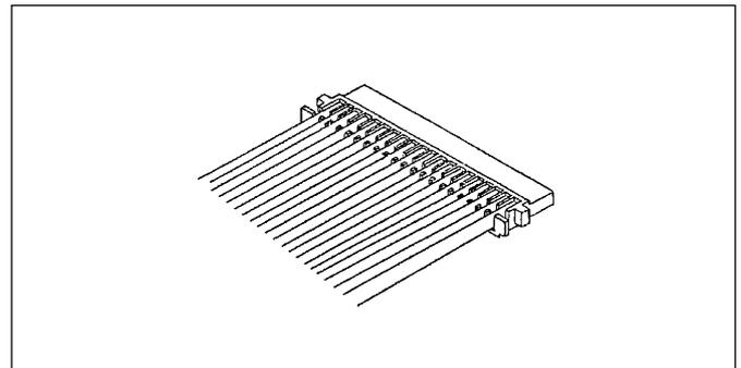
This completes the insulation displacement procedure.
