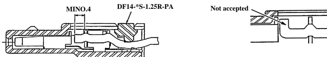
The cable has to jut out by 0.4 mm or more from the insulated portion on the contact point side.
