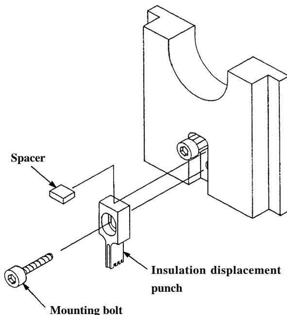
Product number of HRS number of the Insulation displacement punch are as follows:
