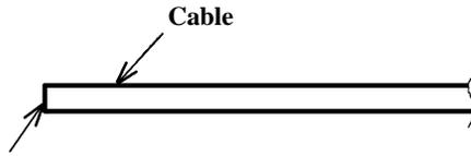
Cut the cable to finish a vertical cut surface.
