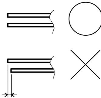
Cut ends of cables are not flush with each other.
