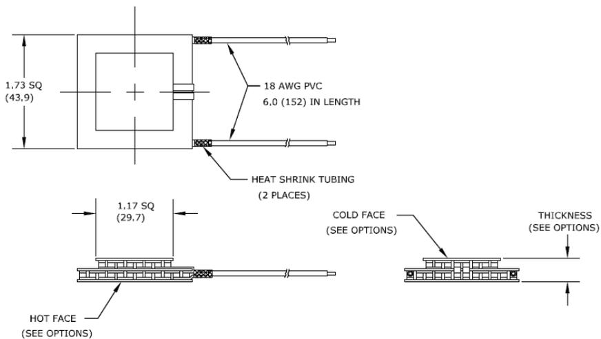
Ceramic Material: Alumina ( $\text{Al}_2\text{O}_3$ )
