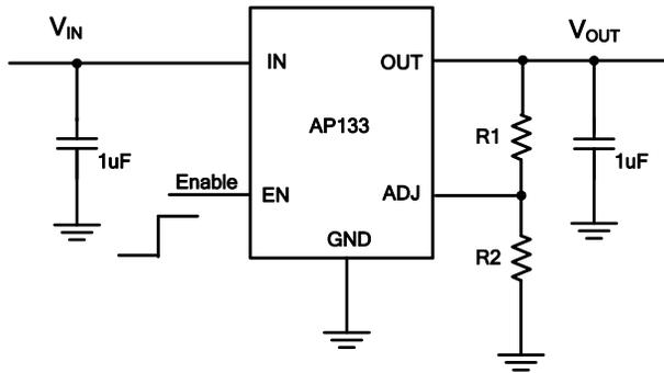
$$V_{OUT} = V_{REF} \left( 1 + \frac{R_1}{R_2} \right)$$
