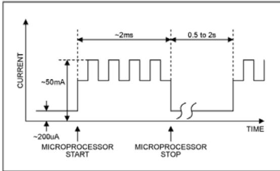
In the standby mode, the microprocessor consumes only around 200µA. Since the phone stays in standby for the longest percentage of time, using a 40µA quiescent current LDO, instead of 140µA, saves 100µA and extends the standby time by 340µA/240µA, or 1.417 times.
