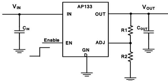
The output voltage is calculated by:
