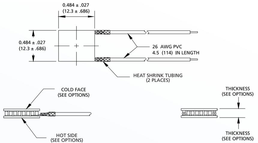
Ceramic Material: Alumina ( $\text{Al}_2\text{O}_3$ )
