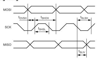
Table 23-8. Serial Programming Characteristics,  $T_A = -40^{\circ}$ C to +125°C,  $V_{CC} = 2.7 - 5.5$ V (Unless Otherwise Noted)
