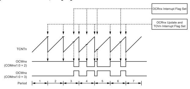
The Timer/Counter overflow flag (TOV1) is set each time the counter reaches TOP. If the interrupt is enabled, the interrupt handler routine can be used for updating the compare value.
