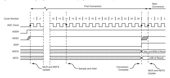
Figure 19-5. ADC Timing Diagram, Single Conversion
