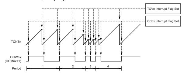
The Timer/Counter overflow flag (TOV1) is set in the same clock cycle as the TCNT1 becomes zero. The TOV1 flag in this case behaves like a 11th bit, except that it is only set, not cleared. However, combined with the timer overflow interrupt, that automatically clears the TOV1 flag, the timer resolution can be increased by software. There are no special cases to consider in the normal mode, a new counter value can be written anytime.
