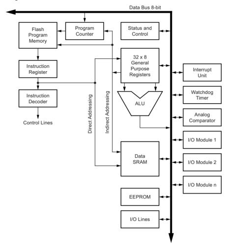
In order to maximize performance and parallelism, the AVR uses a Harvard architecture – with separate memories and buses for program and data. Instructions in the program memory are executed with a single level pipelining. While one instruction is being executed, the next instruction is pre-fetched from the program memory. This concept enables instructions to be executed in every clock cycle. The program memory is in-system reprogrammable flash memory.
