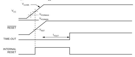
Figure 9-3. MCU Start-up, RESET Extended Externally
