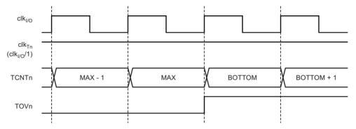
Figure 14-6 shows the same timing data, but with the prescaler enabled.
