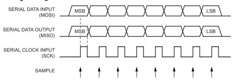
Figure 23-7. Serial Programming Timing
