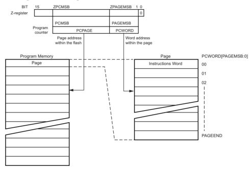
1. The different variables used in Figure 21-1 are listed in Table 22-7 on page 159. Note:
