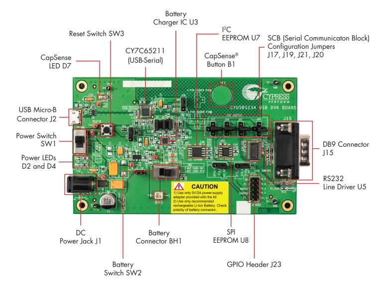
Note: By default, the SCB configuration jumpers are set for the USB-UART bridge as shown above. Refer to the Table 3-1 in the kit guide for additional information on default jumper settings.
