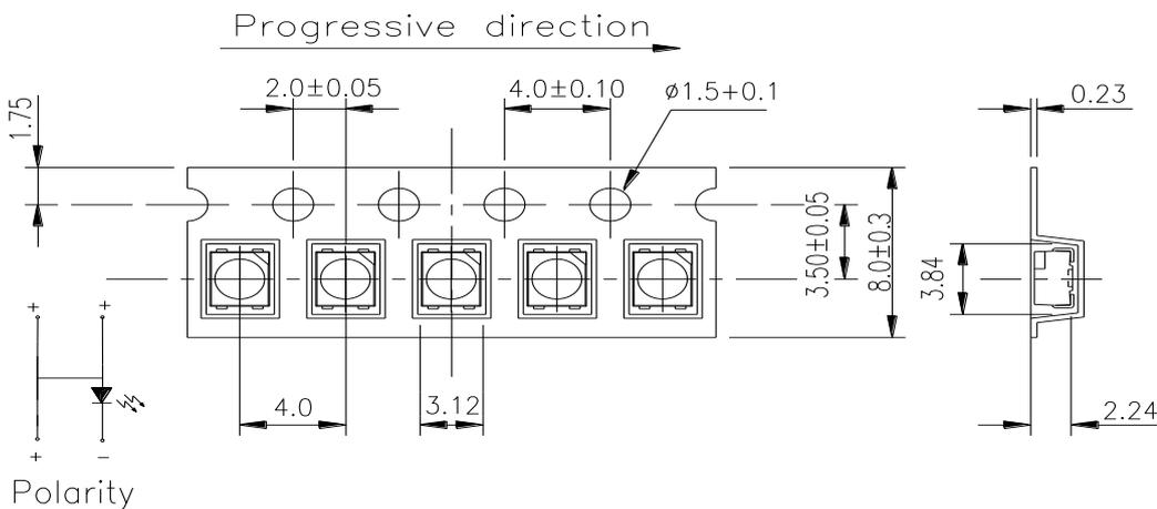
Note: Tolerances unless mentioned  $\pm 0.1$ mm. Unit = mm
