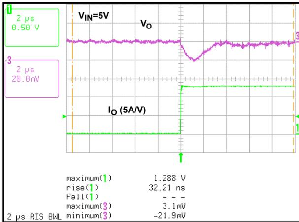
FIGURE 8. STEP-UP TRANSIENTS AT NO LOAD ( $V_{IN} = 5.0V$ )
