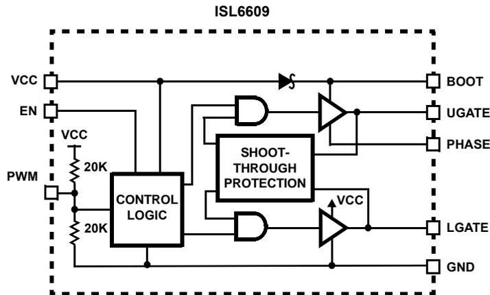
FIGURE 2. SIMPLIFIED ISL6558 AND ISL6609 INTERNAL STRUCTURE
