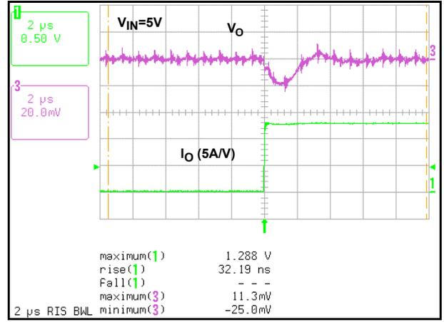
FIGURE 11. STEP-UP TRANSIENTS AT 25A ( $V_{IN} = 5.0V$ )
