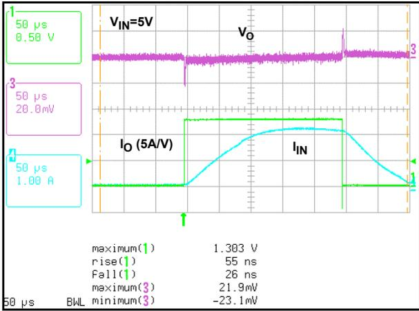
FIGURE 7. TRANSIENT RESPONSE AT NO LOAD ( $V_{IN} = 5.0V$ )
