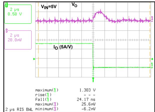
FIGURE 12. STEP-DOWN TRANSIENTS AT 25A ( $V_{IN} = 5.0V$ )
