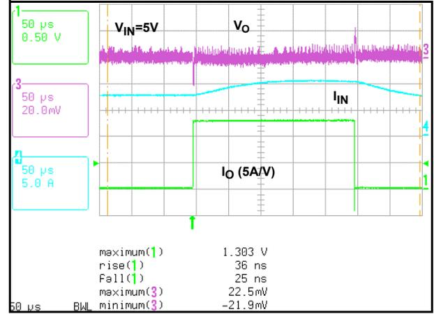
FIGURE 10. TRANSIENT RESPONSE AT 25A ( $V_{IN} = 5.0V$ )
