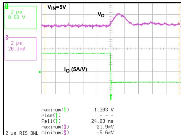
FIGURE 9. STEP-DOWN TRANSIENTS AT NO LOAD ( $V_{IN} = 5.0V$ )
