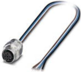
Sensor/actuator flush-type socket, 4-pos., M12 SPEEDCON, A-coded, front/screw mounting with M16 thread, can be positioned, with 1 m TPE litz wire, 4 x 0.34 mm<sup>2</sup>
