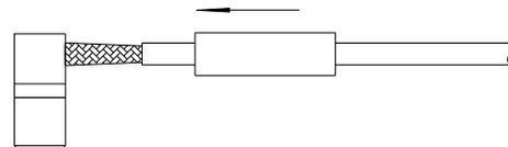
7. CRIMP OUTER FERRULE WITH APPROPRIATE CRIMP TOOL.
