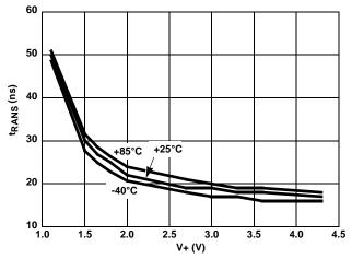
FIGURE 13. ADDRESS TRANS TIME vs SUPPLY VOLTAGE
