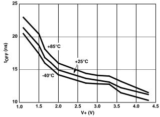
FIGURE 15. INHIBIT TURN-OFF TIME vs SUPPLY VOLTAGE
