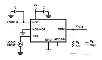
Repeat test for other switches. CL includes fixture and stray capacitance.  $$\sf R$$
