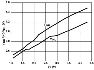
FIGURE 12. DIGITAL SWITCHING POINT vs SUPPLY VOLTAGE
