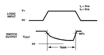
FIGURE 3A. t<sub>BBM</sub> MEASUREMENT POINTS
