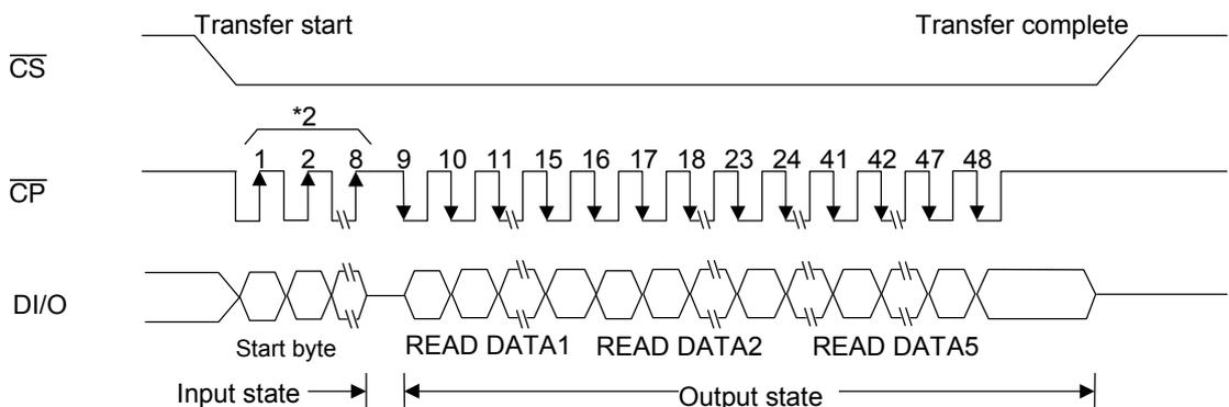
\*2: A reading state appears only when the R/W bit is "1". The read data is valid only when the register is set to key scan read mode and display data read mode. Otherwise, the read data is invalid.
