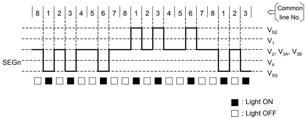
**Liquid Crystal Driving Waveform Example (2)**
