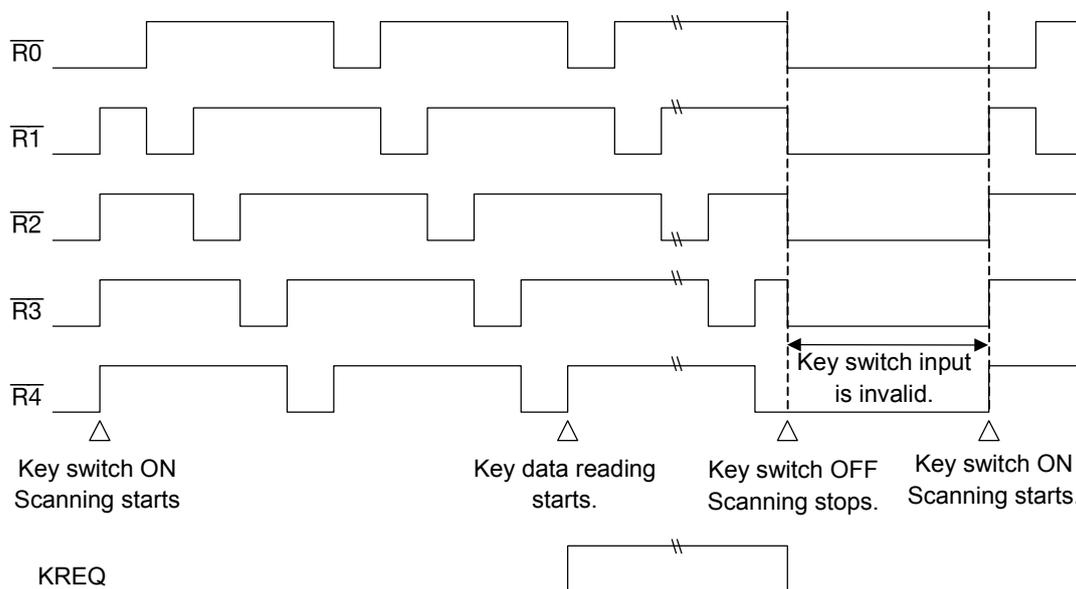
Note 1: When three or more key switches are pressed at the same time, the ML9090A-01/02 may recognize that an unpressed key switch is pressed. Therefore, to recognize simultaneous depression of three or more key switches, add a diode in series to each key. (See Figure 1.) To ignore simultaneous depression of three or more key switches, a program may be required to ignore all key data which contain three or more consecutive “1” values.
