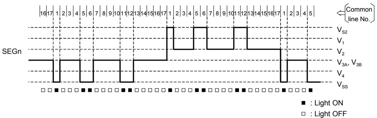
**Liquid Crystal Driving Waveform Example (6)**
