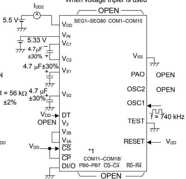
\*1: PB0 - PB7 for ML9090A-01, and COM11 - COM18 for ML9090A-02
