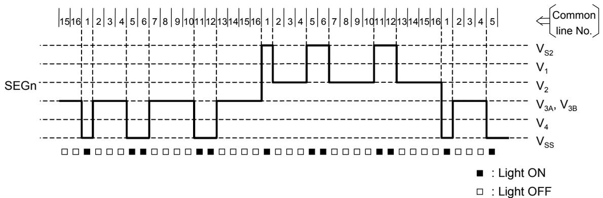
**Liquid Crystal Driving Waveform Example (5)**
