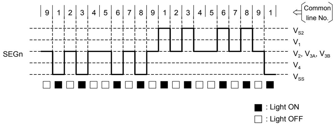
**Liquid Crystal Driving Waveform Example (3)**
