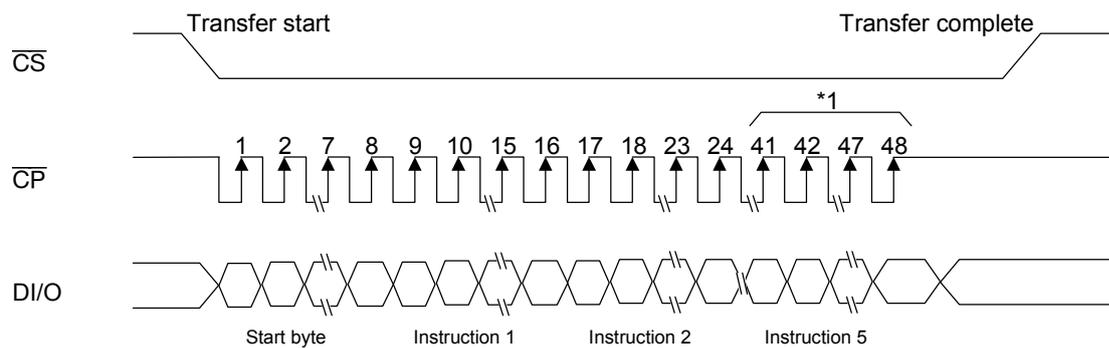
\*1: Write data in 8 bits. If the  $\overline{CS}$  signal falls when data input operation in 8 bits is not complete, the last 8-bit data write is invalid. (The previously written data is valid)
