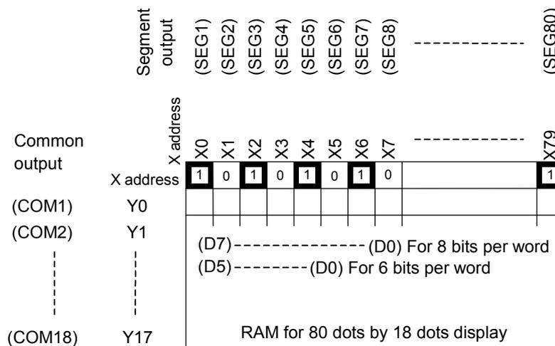
**Figure 3 Display Screen Bit Allocation and Memory Addresses**
