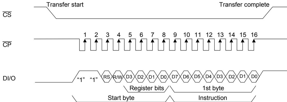
**Clock Synchronous Serial Continuous Data Transfer Example (WRITE)**
