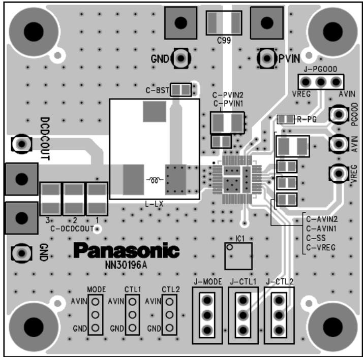
Figure 6. Top Layer with silk screen ( Top View )
