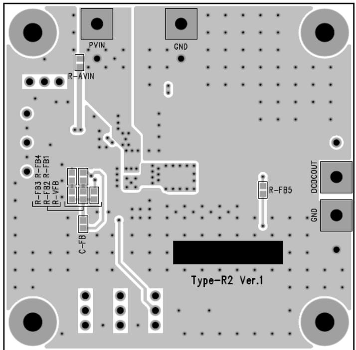
Figure 7. Bottom Layer with silk screen ( Bottom View )
