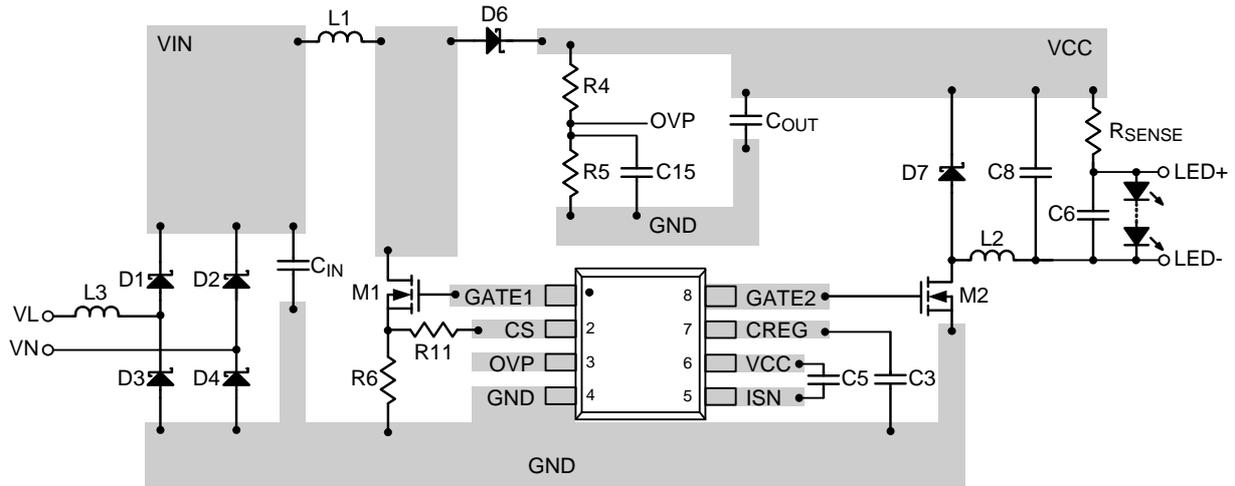
Figure 2. PCB Layout Guide for SOP-8 Package
