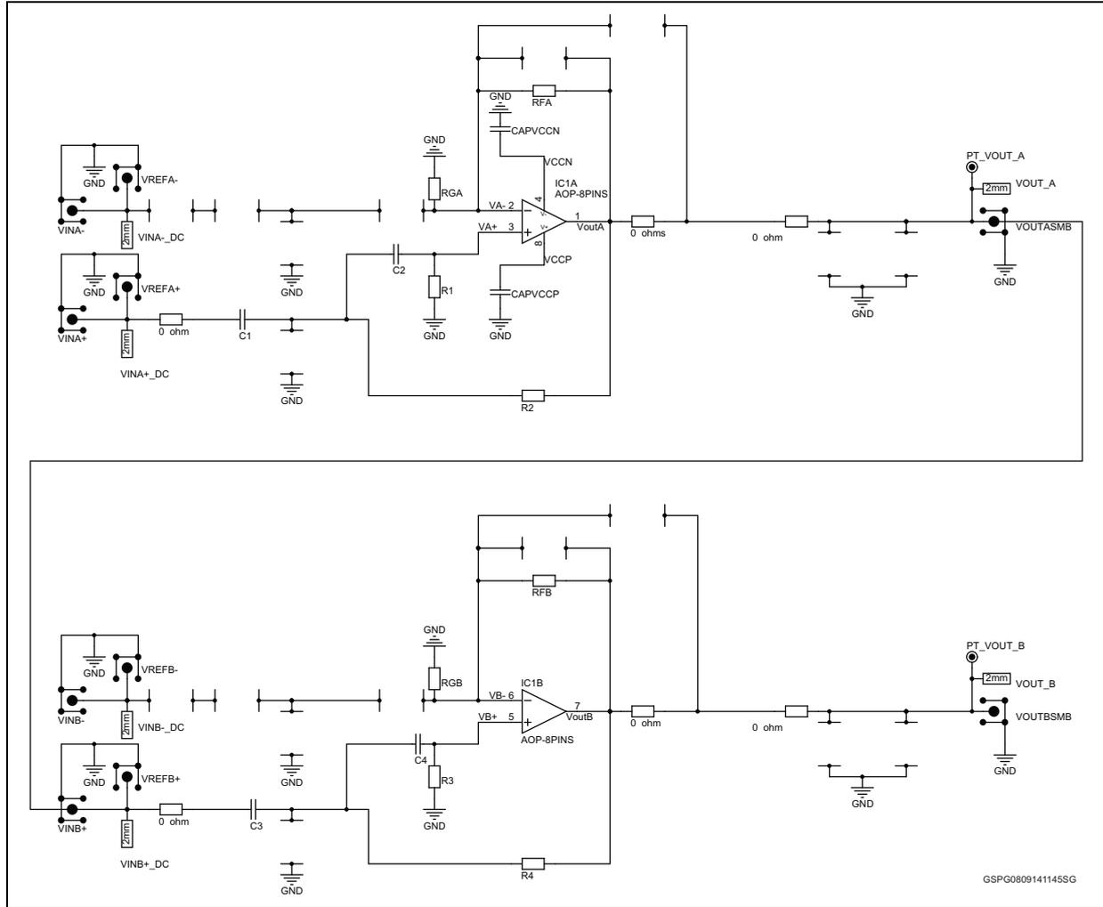
The upper limit of the frequency range is determined by the GBP of the op amp ( $F \ll \frac{GBP}{1 + \frac{R_F}{R_G}}$ )
