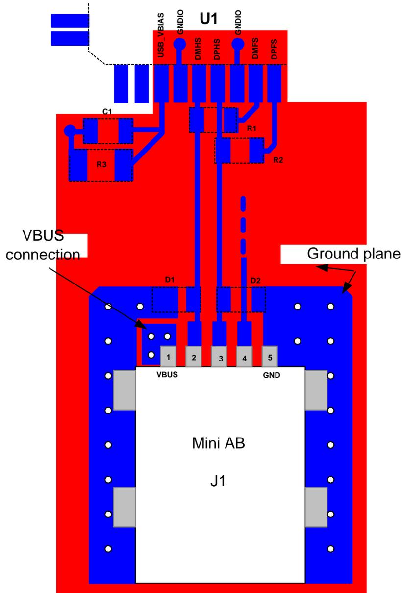
Figure 3-2. Standard Mini AB Receptacle - USB Routing Example with BGA144 Package
